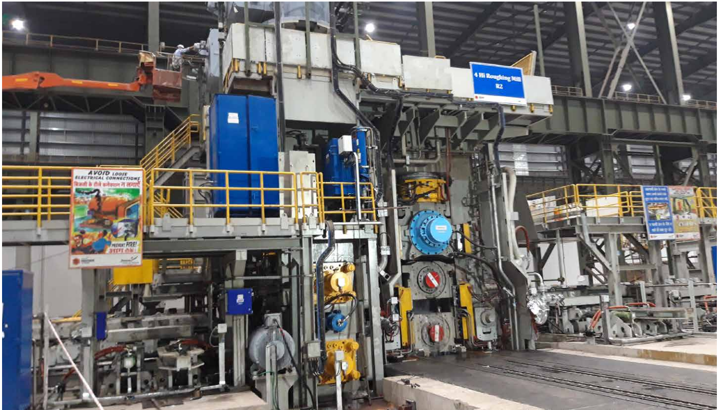
Roughing mill No. 2 in 4 hi-design with attached edger (Picture: SMS group)
