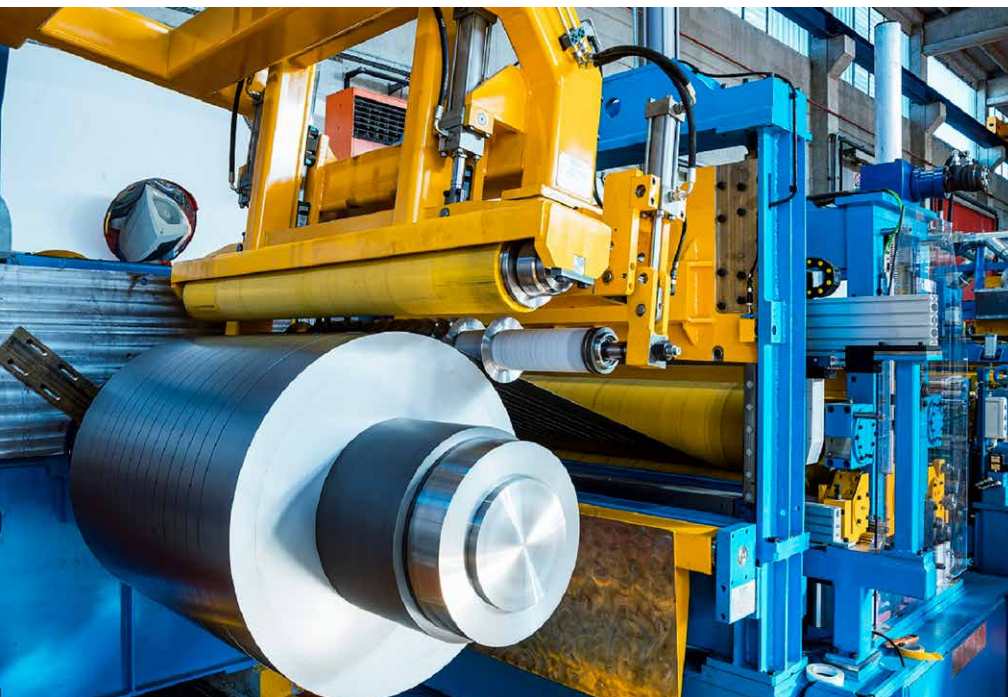
New slitting line to meet the increased demand for high-quality electrical steel
