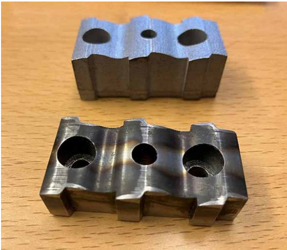
At the top a 3D-printed blank and the part below it is a finished and laser-hardened stamp after use in production (Picture: SSAB)
