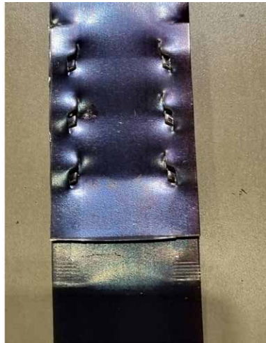
Punched strap (left) and the locking mechanism (right) with stamp, 3D printed and laser hardened (Picture: SSAB)
