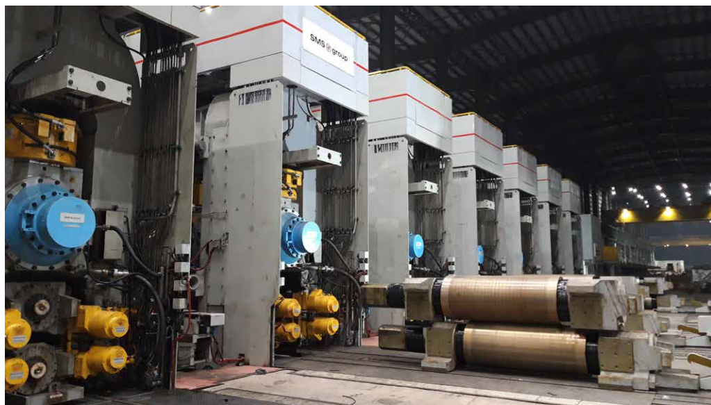
Seven finishing mill stands are equipped with latest generation actuators (Picture: SMS group)
