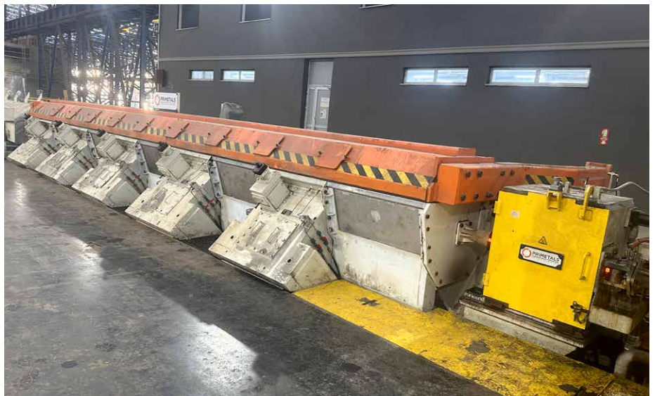
10-stand next-generation Morgan No-Twist mill (Picture: Primetals Technologies.)
