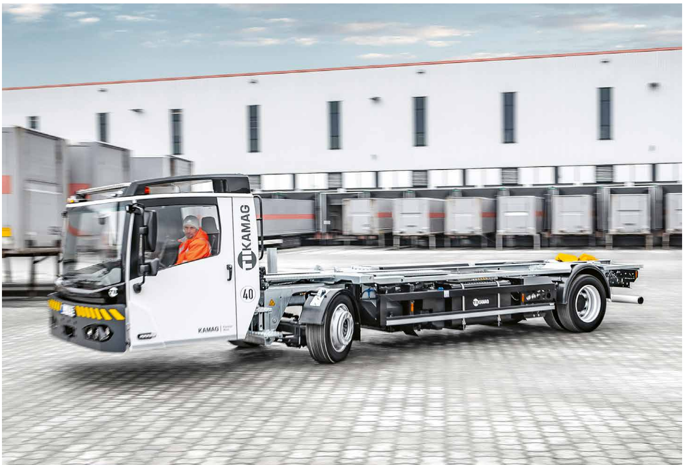
The galvanised frame, lifting table and cab mounting system provides the KAMAG PrecisionMover with reliable corrosion protection (Photo: TII Group)
