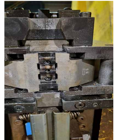
Punched strap (left) and the locking mechanism (right) with stamp, 3D printed and laser hardened (Picture: SSAB)
