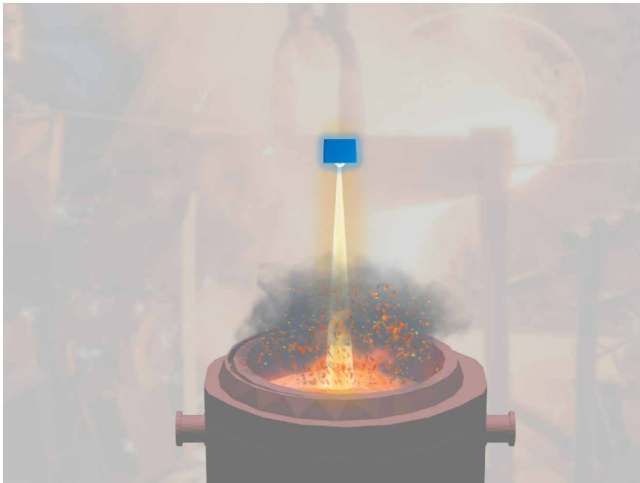
Schematic of radar level measurement in a crucible (Picture: OndoSense)
