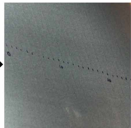
Example of marks on strip surface due to 5th Octave Chatter → product not saleable!
