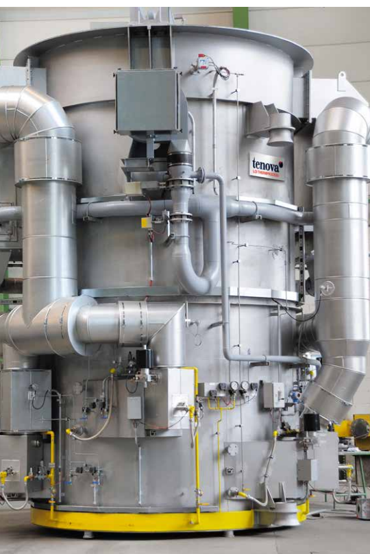
Ultra-low NO x HPH® Flameless heating hood of the bell-type annealing plant at thyssenkrupp Hohenlimburg (Picture: LOI Thermprocess)
