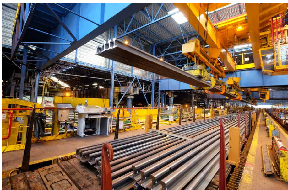
Rails prepared for final inspections and finishing (Picture: Saarlühl Rail Hayange)
