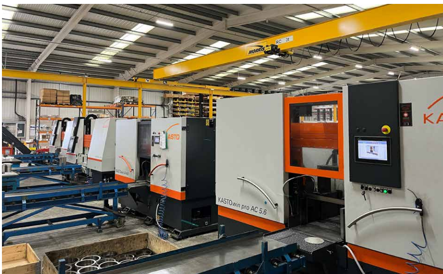
Metal distributor Langley Alloys relies on band saws from Kasto for the machining of difficult-to-cut alloys (Picture: Kasto Maschinenbau)
