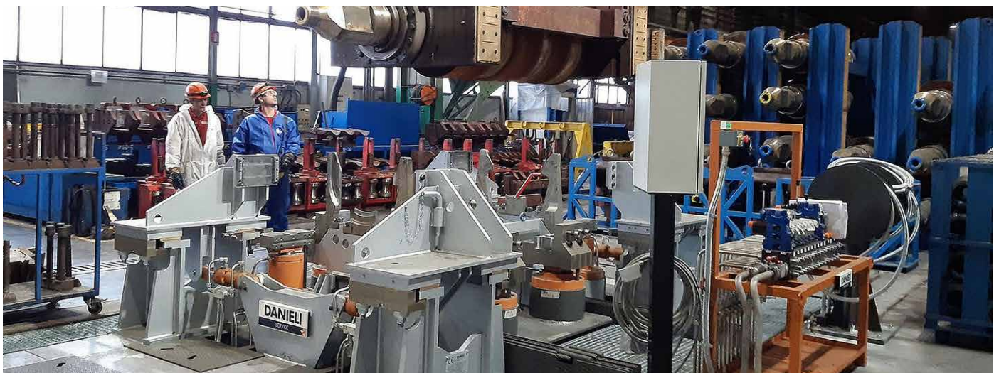
This new device makes the assembly and disassembly of work roll arrangement safer, faster and more precise (Picture: Danieli)
