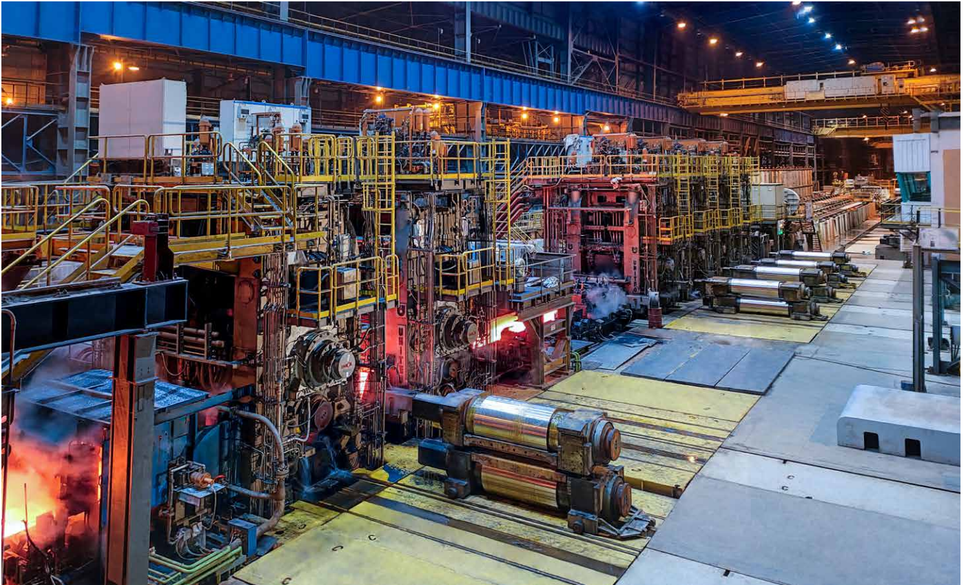
Rolling mill in 2 + 4 stand configuration with the option for possible installation of a fifth finishing stand (Picture: Danieli)
