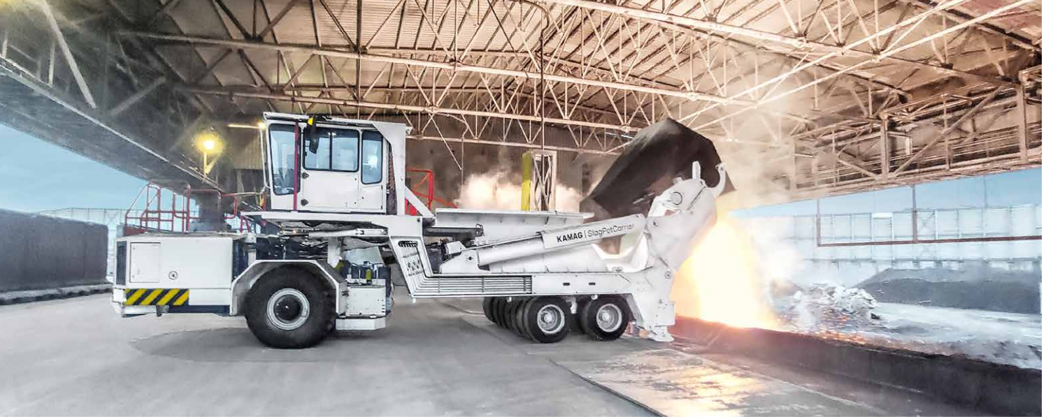
Slag pot carrier operated by Harsco at a steelmaker in Brescia, Italy (Picture: TII Group)
