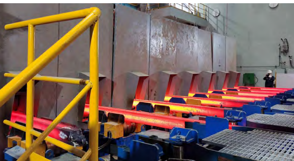
The billet caster produces quality 220-mm-square and up to 250-mm-round products on eight strands (Picture: Danieli)
