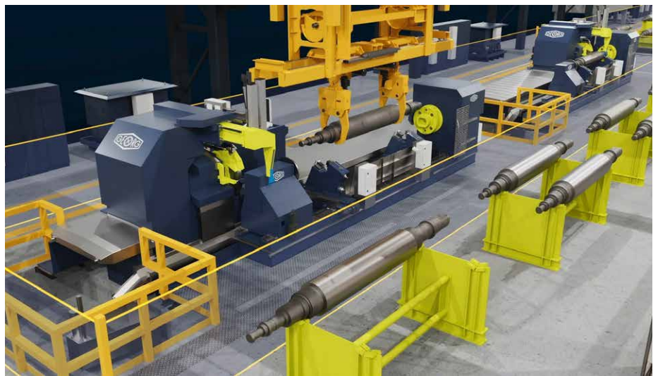
“ultragrind10” grinding machines are charged by a semi-gantry loader (yellow) (Picture: GEORG)
