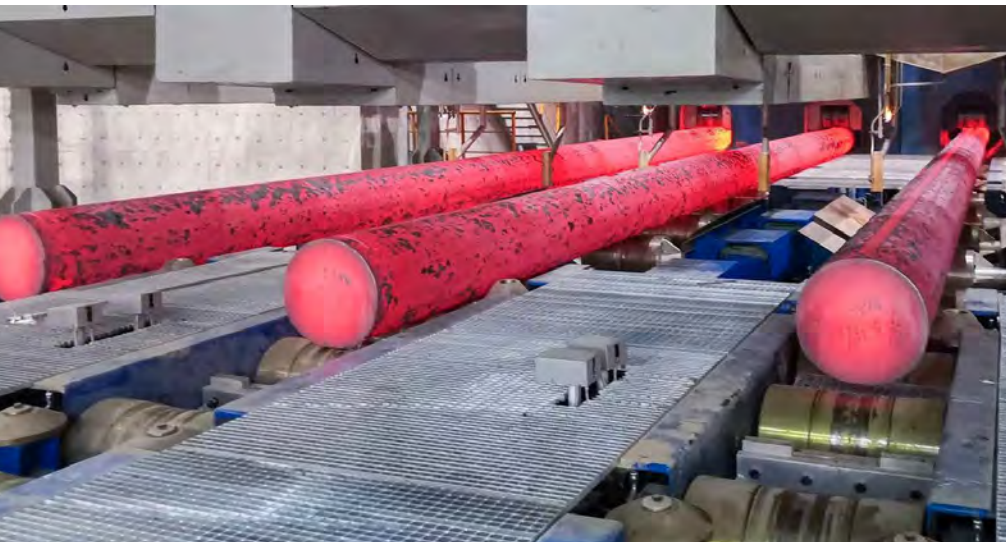
The four-strand jumbo caster can produce blooms of diameter 600 to 1200 mm (Picture: Danieli)
