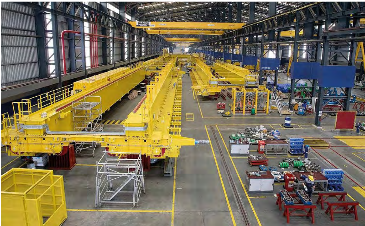
The intelligent cranes have been manufactured at the workshops of Danieli Thailand (Picture: Danieli)
