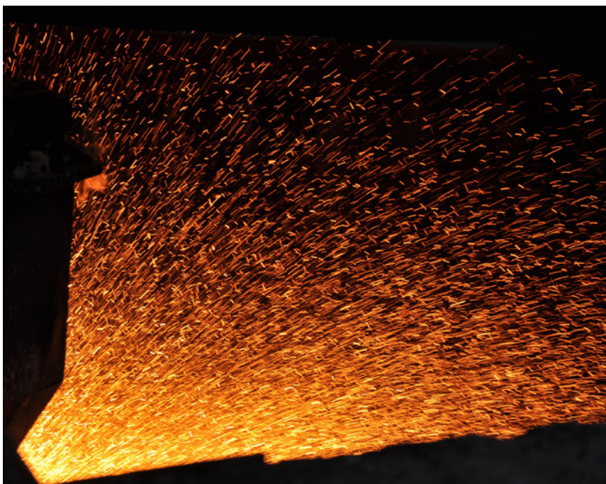
In the induction furnaces, stainless steel is melted and then atomized, creating the spherical CHRONITAL.
