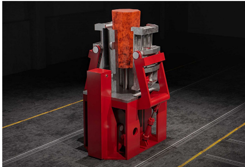
Block pusher with sectional view of filled ingot mold. Photo: Dango & Dienenthal Maschinenbau GmbH
