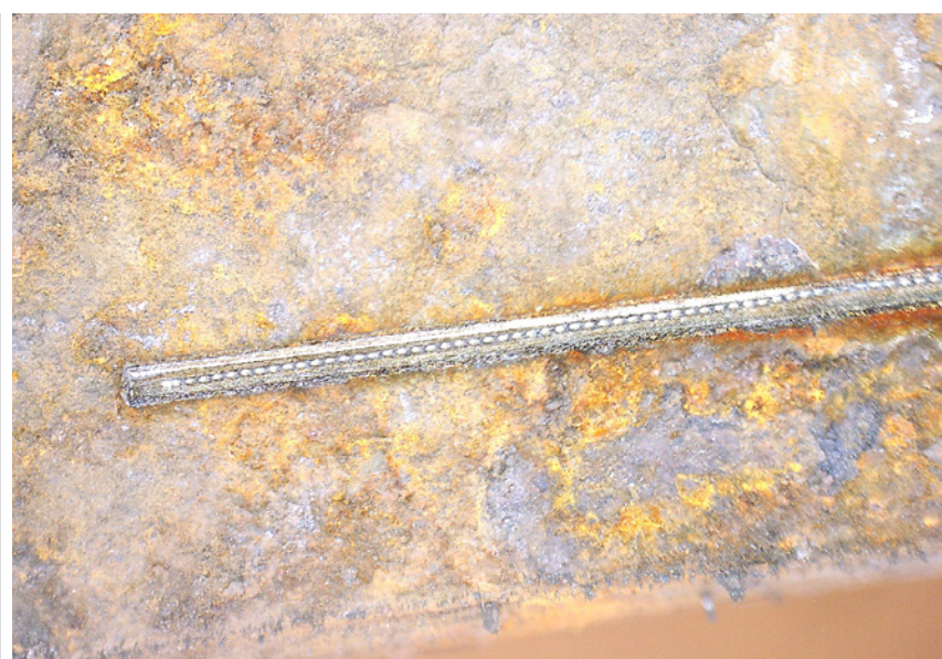
FiberLIBS removes oxide, carbonization and scale deposits from the billet surface by laser ablation, before it starts the LIBS measurement.
