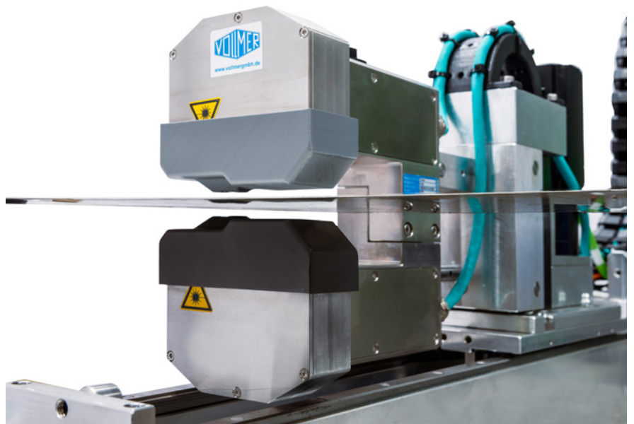
The VTLG 101/1 for laser-based thickness measurement on foils with thicknesses between 0.003 and 2.0 mm is so compact that it can be installed in the immediate vicinity of the roll gap.
