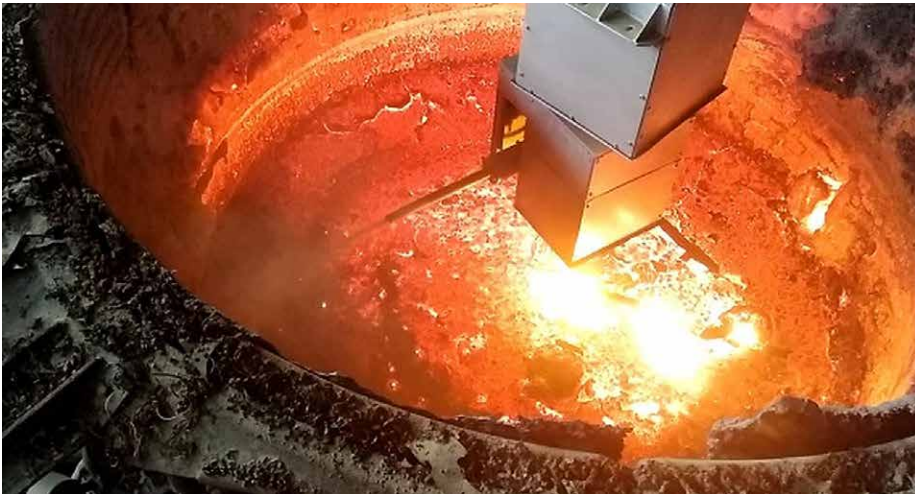
EAF ginning robot Hytop during operation (Picture: VELCO)
