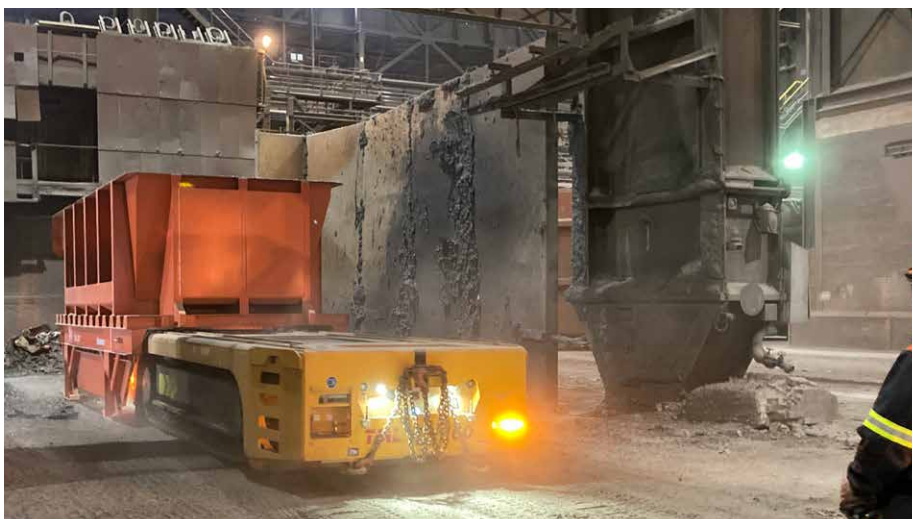
Remotely controlled, the Hot Box Mover positions the Hot Box under the furnace (Picture: TML)
