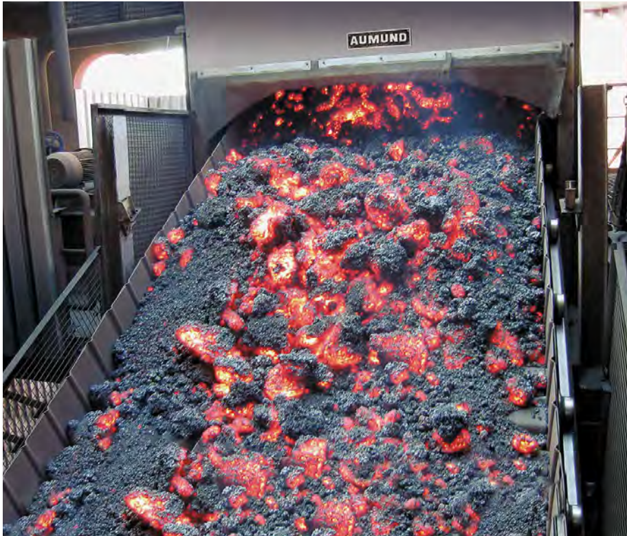
Aumund pan conveyor type KZB-S in a sintering plant (Picture: Aumund)
