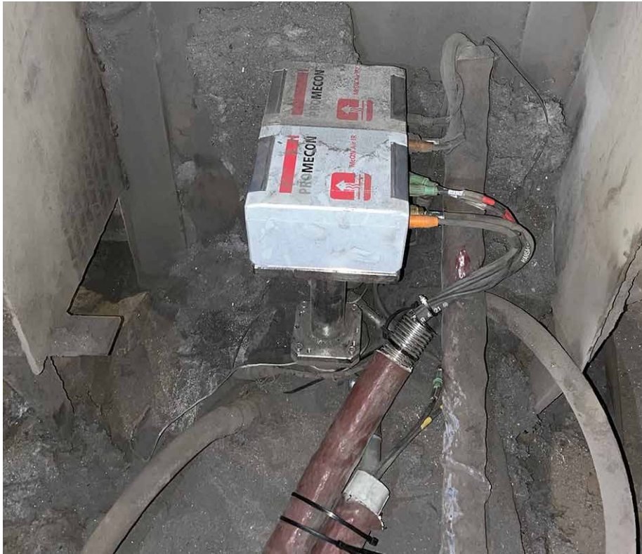
Outer parts of the sensors applied at the EAF of FERALPI STAHL in Riesa, Germany (Picture: PROMECON)
