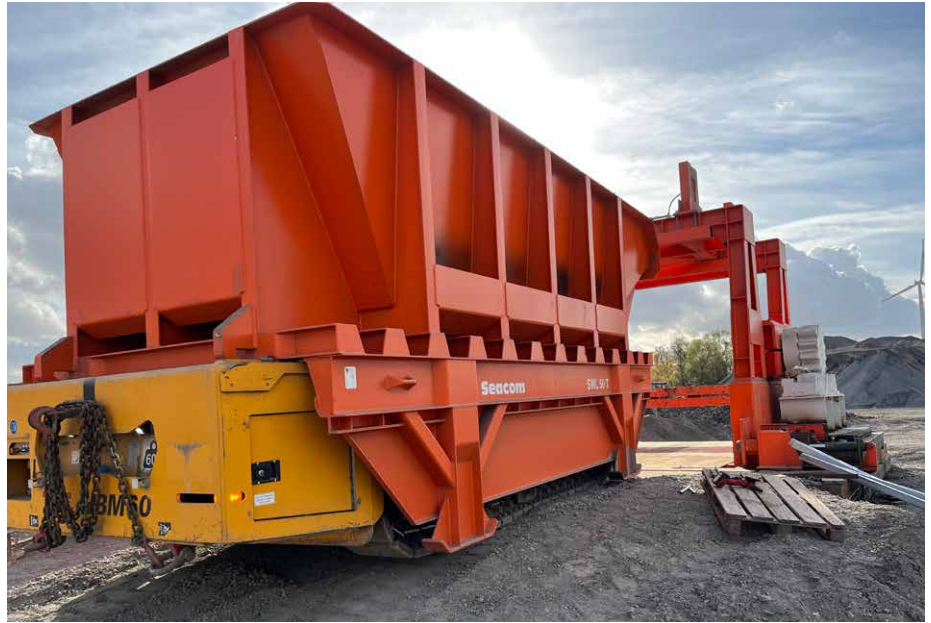
Hot Box Mover with Hot Box entering the tipping device (Picture: TML)
