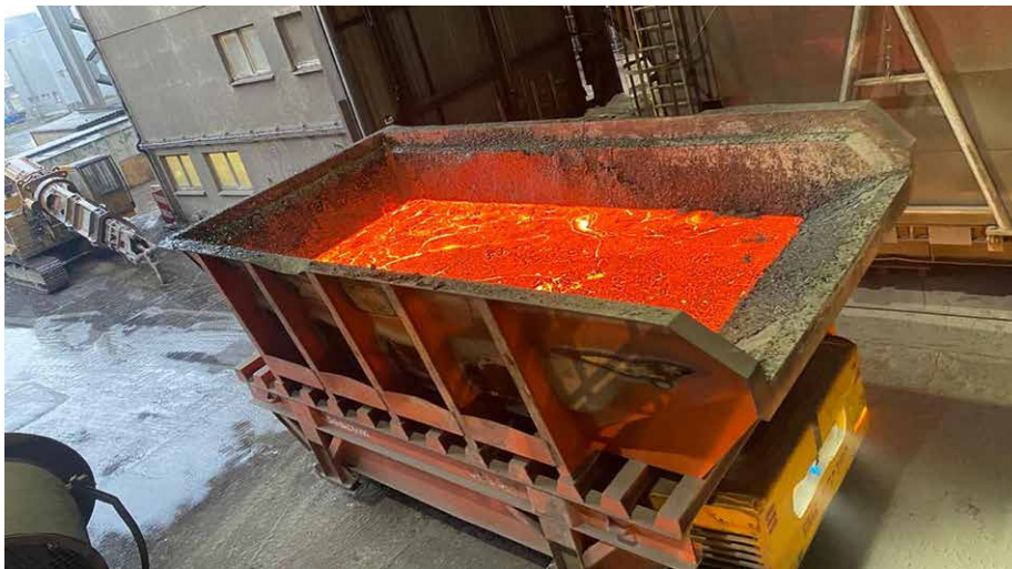
Hot Box filled with liquid slag leaving the steel plant on a Hot Box Mover (Picture: TML)
