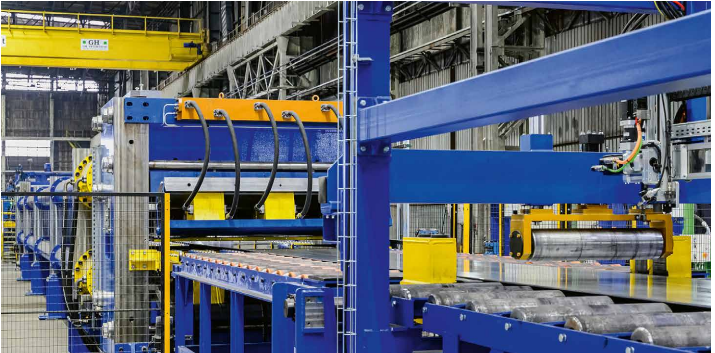
AMDS Kraków can produce Armstrong® sheets with a maximum deviation of just three millimetres per metre (Picture: Kamil Pyzynski/ ArcelorMittal)
