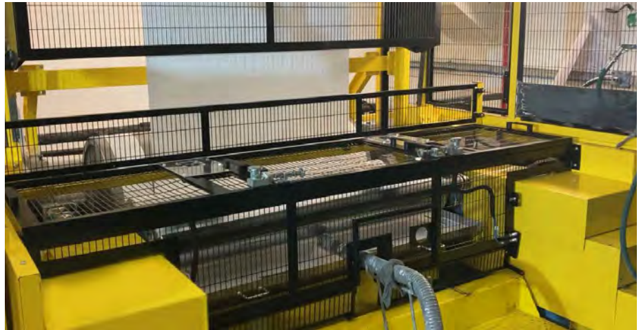
New coater head for Tata Steel's Shotton works (Photo: Tata Steel)
