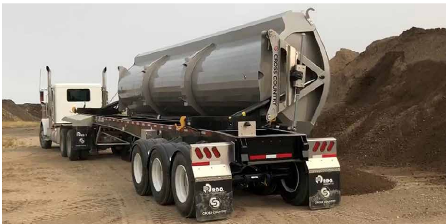
Cross Country Manufacturing in Manitoba, Canada, side tipper model increased profitability with Strenx® steel due to higher payloads and lower fuel consumption
