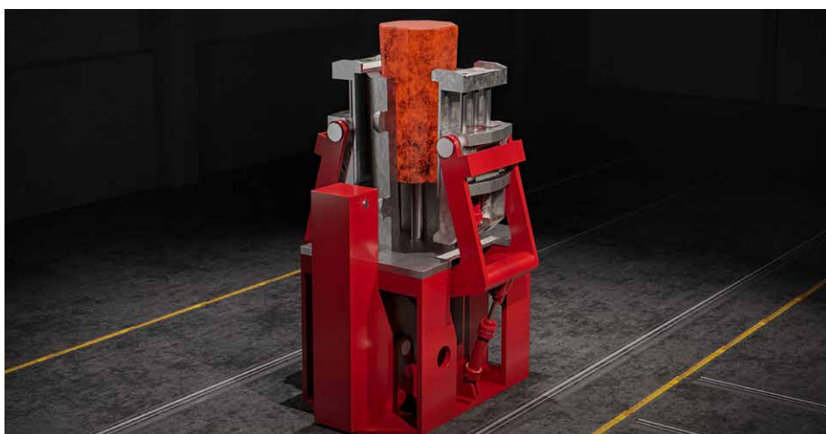
Block pusher with sectional view of filled ingot mold (Picture: Dango & Dienenthal)
