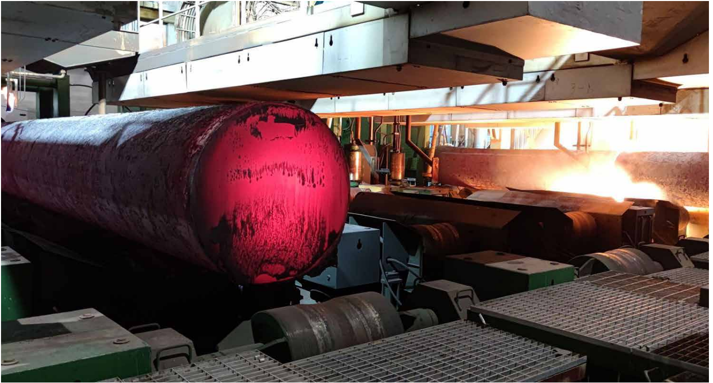
Dia. 1,200 mm round bloom casting at Jiangsu YongGang (Picture: Danieli)
