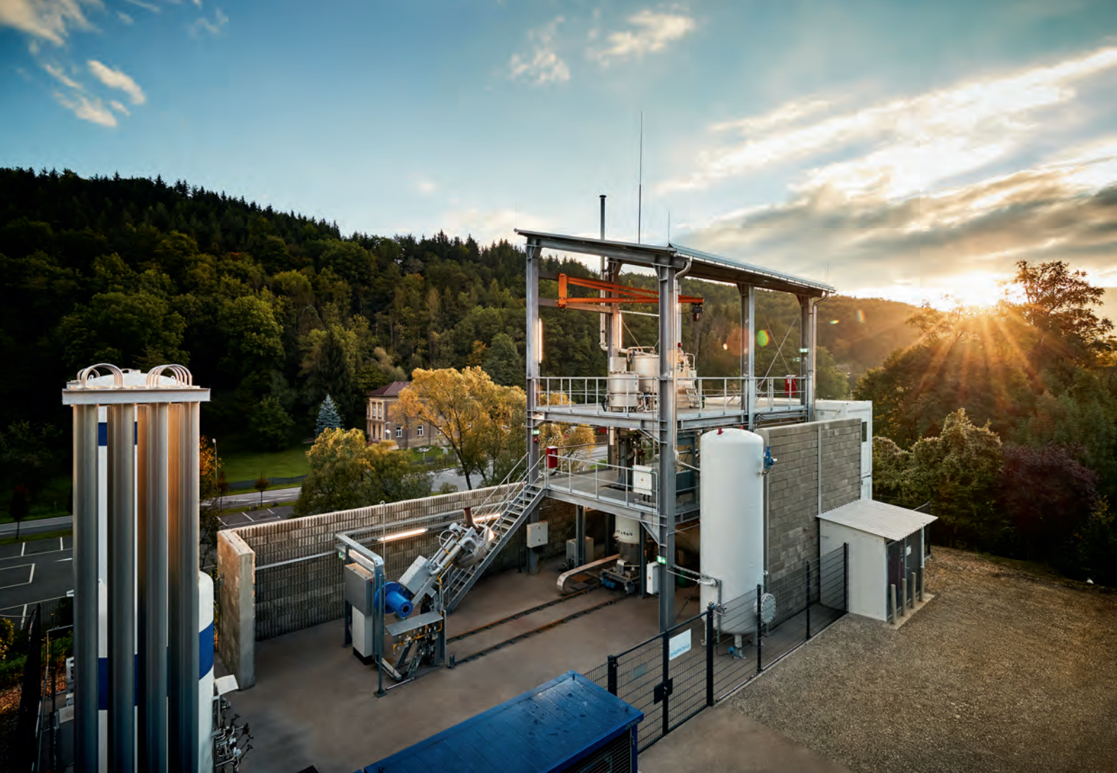
The CO 2 -free production of liquid steel in hydrogen plasma is being researched in the pilot facility (Picture: voestalpine)
