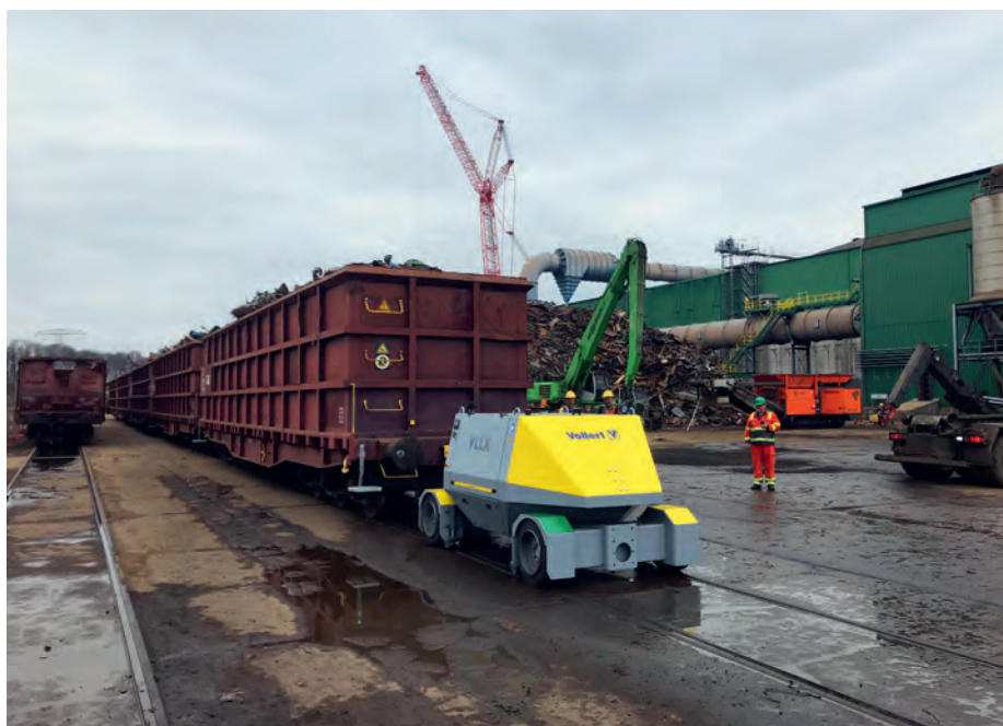
At ESF the VLEX 40 handles the shunting of rail cars weighing up to 600 tons (Picture: Vollert)
