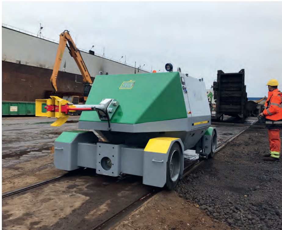
The VLEX 40 road-rail robot is equipped with a camera system for convenient remote control (Picture: Vollert)
