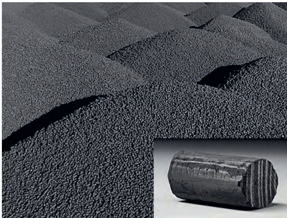
Biocarbon is engineered to immediately displace fossil fuel-based inputs – such as coal or coke in steel and metals production – without the need for any plant modification (Picture: Aymium)
