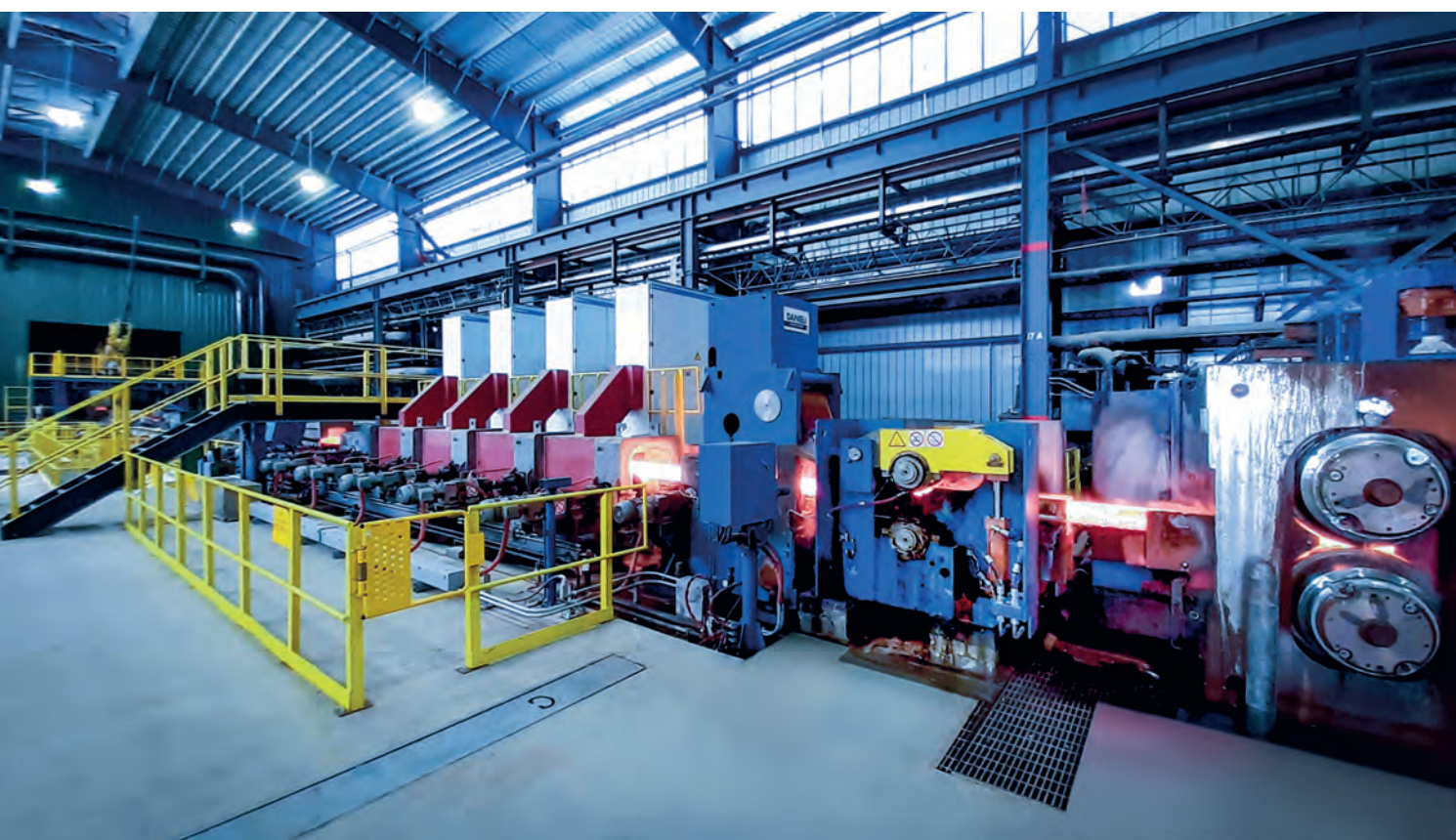
MIDA QLP endless casting technology was developed to run 23.5 hours without changes at the caster (Picture: Danieli)
