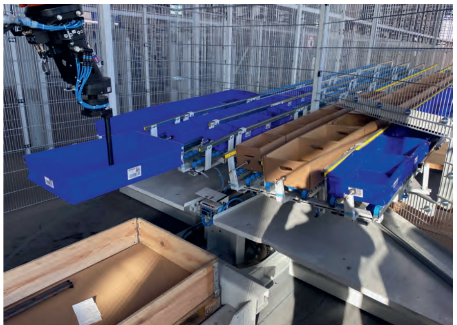
Based on the order data, KASTOsort determines the suitable container for the respective workpieces (Picture: KASTO)
