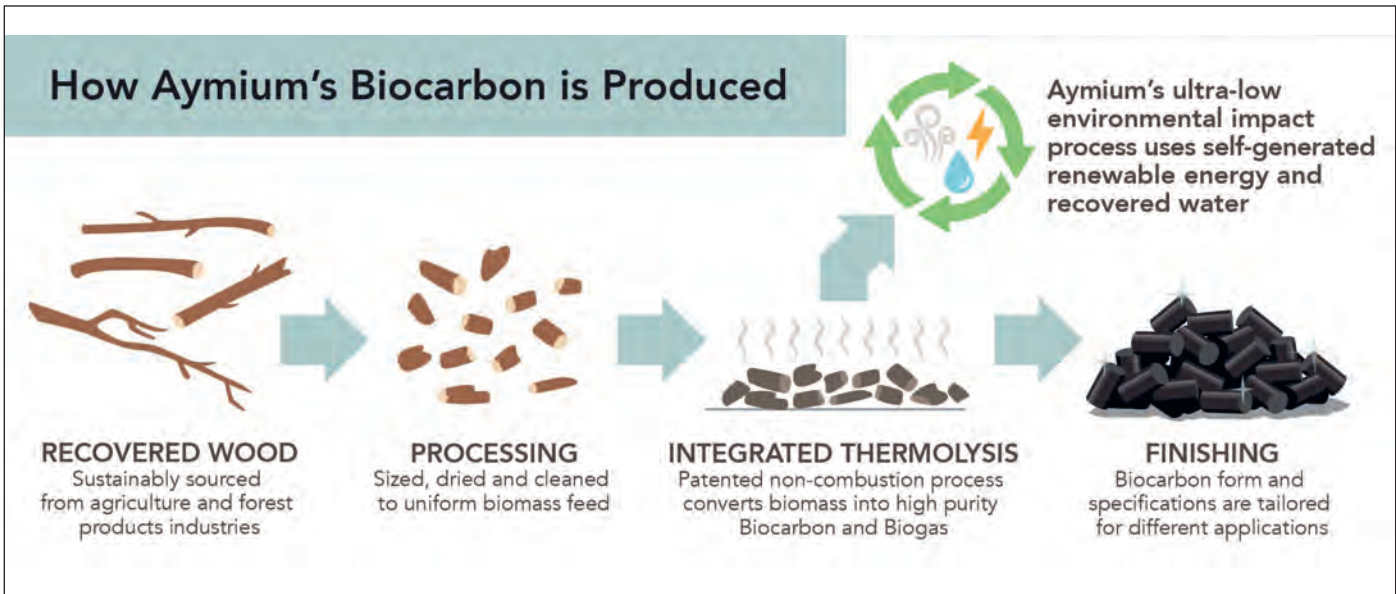
The patented process converts certified sustainably sourced biomass into biocarbon using integrated thermolysis (Picture: Aymium)
