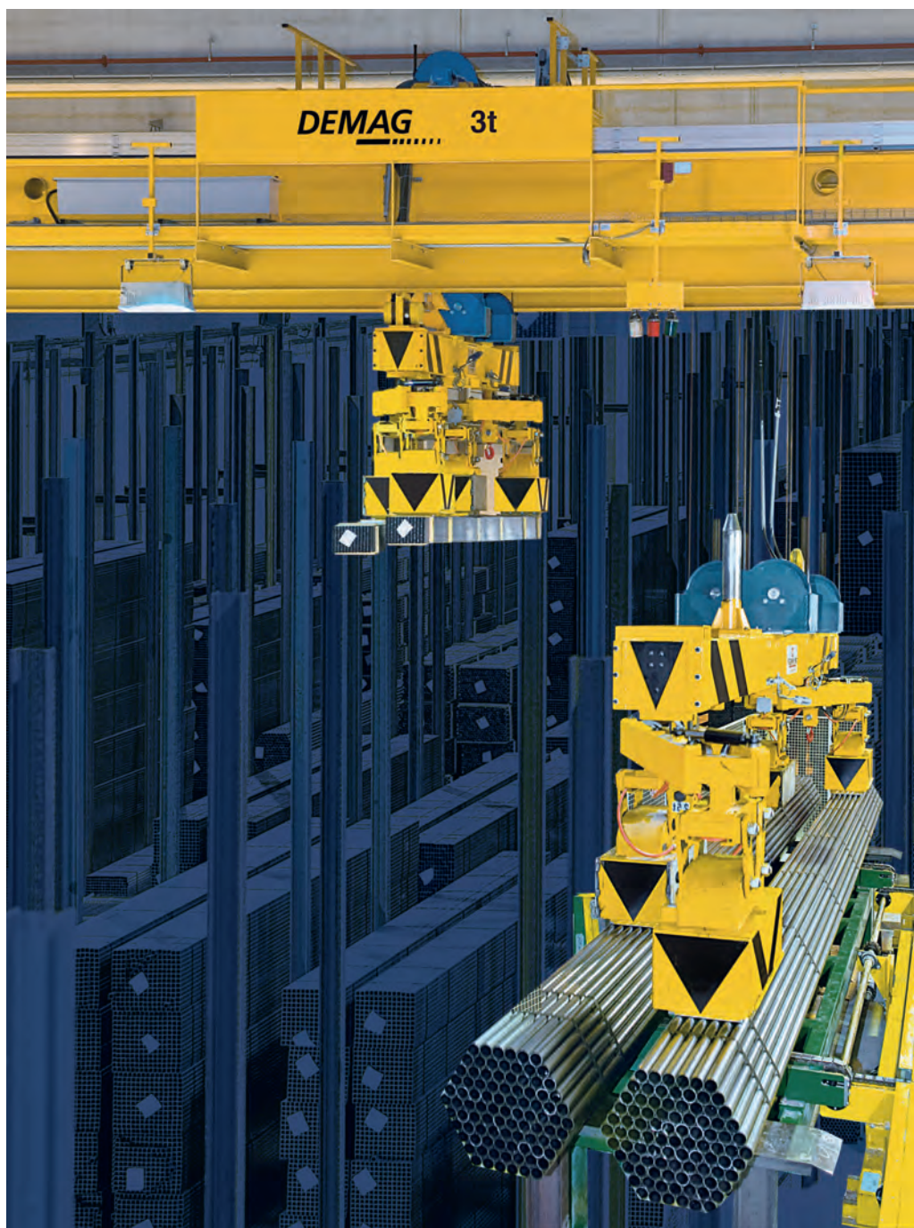
The tubes will be effectively stored, picked and supplied on time for the production of components for scaffolding, with a very high degree of automation
