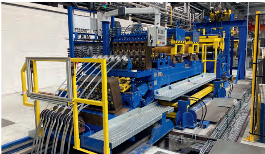
Arrondising plant at Wuppermann Hungary (Picture: Wuppermann)
