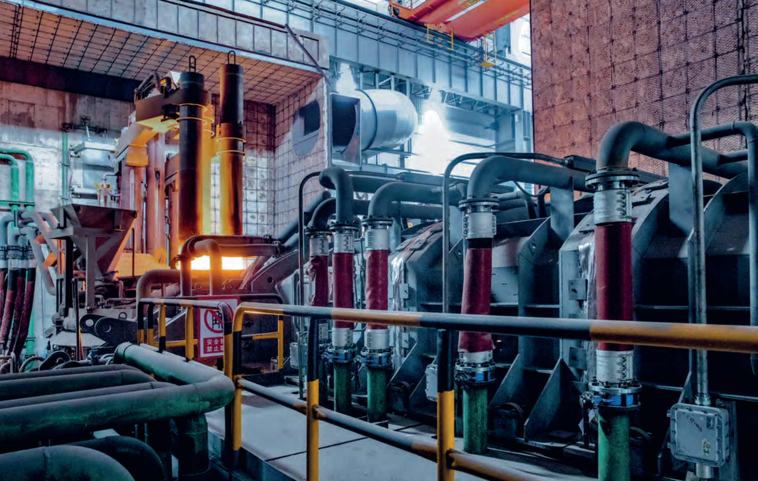
Using the Danieli Digital Melter, which is an advanced EAF, together with the BOF, means that the downstream process route remains the same (Picture: Danieli)
