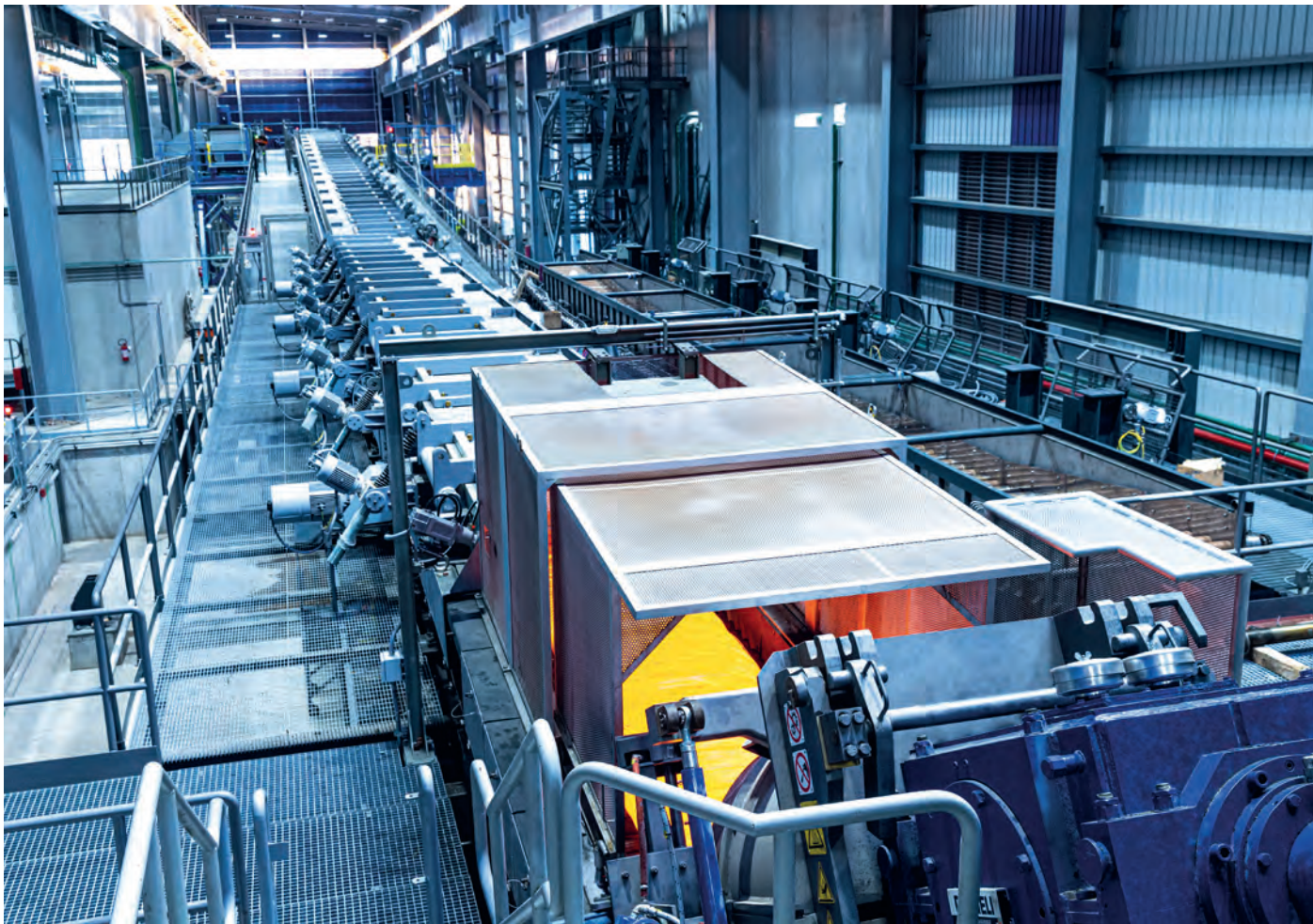
In terms of quality wire rod – QWR, Danieli has developed a rolling mill that is fully electric, fully automatic and fully digital (Picture: Danieli)
