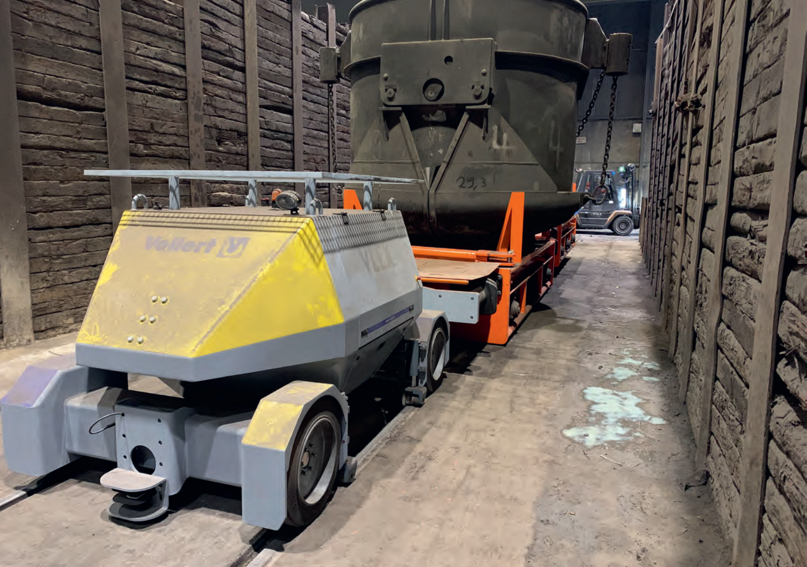
At VDM Metals the road-rail robot VLEX 20 automatically moves a 50-ton bucket charged with scrap to the meltshop (Picture: Vollert)
