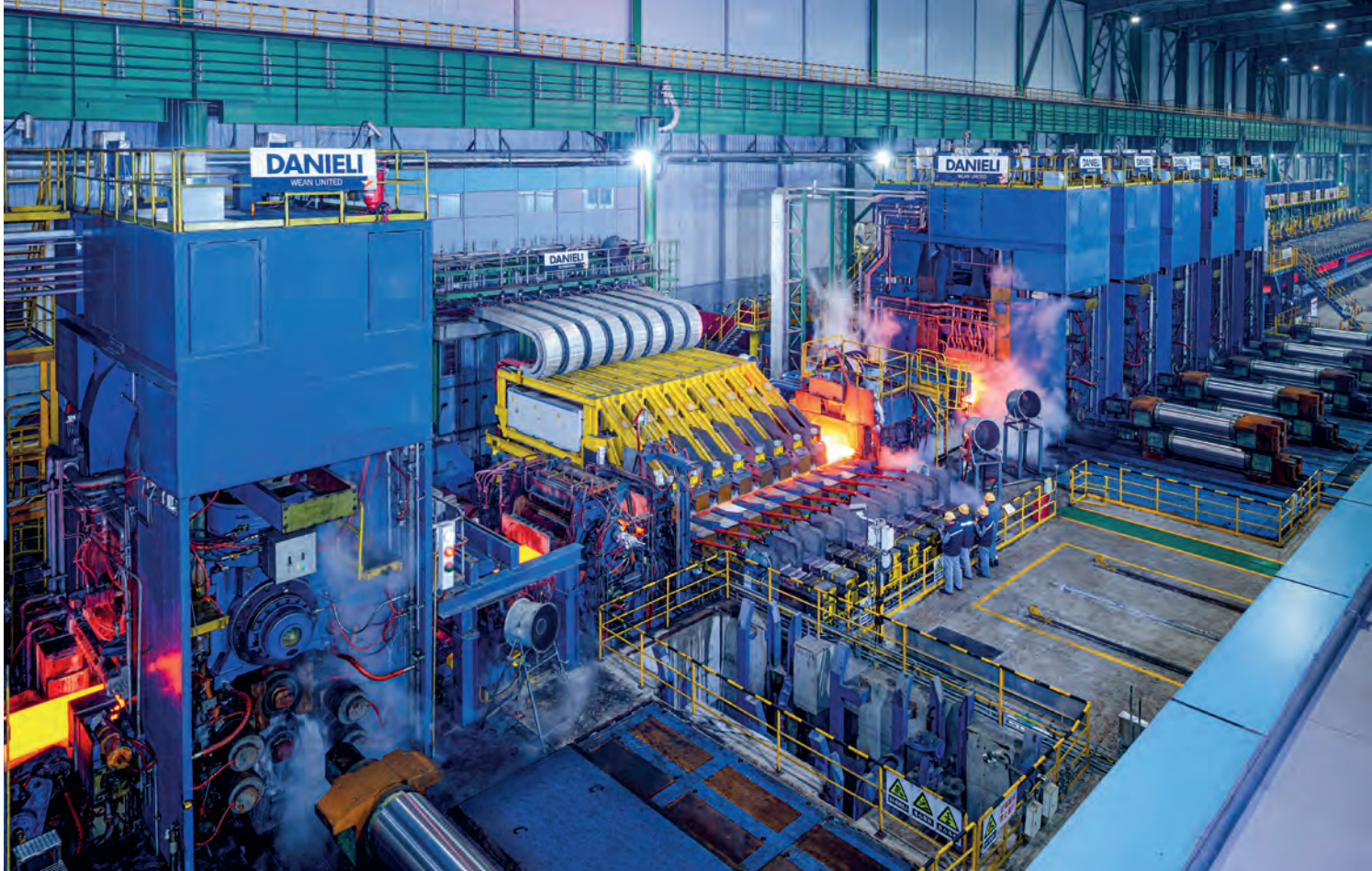
DUE – Danieli Universal Endless technology is now recognized an eco-friendly way to produce thin hot strip in the thickness range of 1.5 mm (Picture: Danieli)
