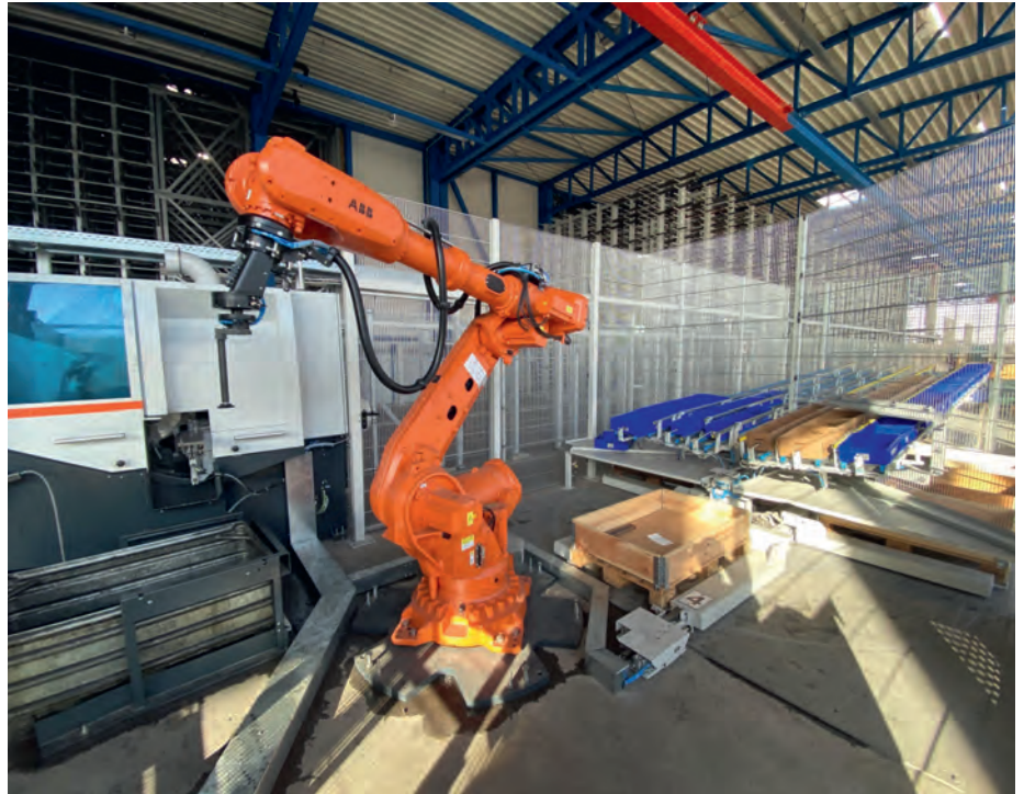
A robot places the required boxes on a pallet provided with the help of a suction device and fills them with cut-pieces (Picture: KASTO)
