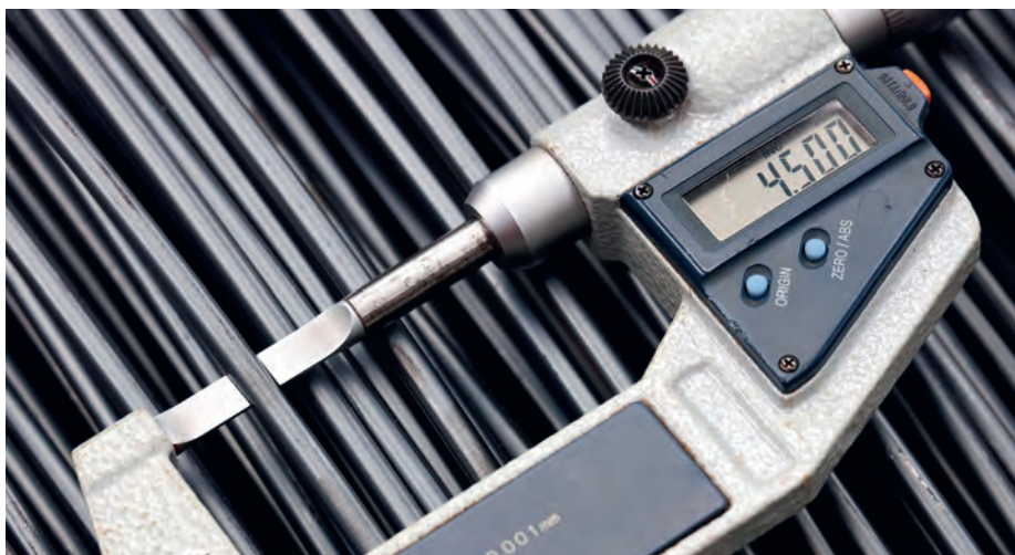
The 4.5 mm wire rod is produced at the Burbach rolling mill on the four-strand wire rod mill (Picture: Dirk Martin/Saarstahl)
