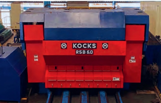
The commissioned reducing & sizing block for bar-in-coil and straight bar production (Photo: Kocks)
