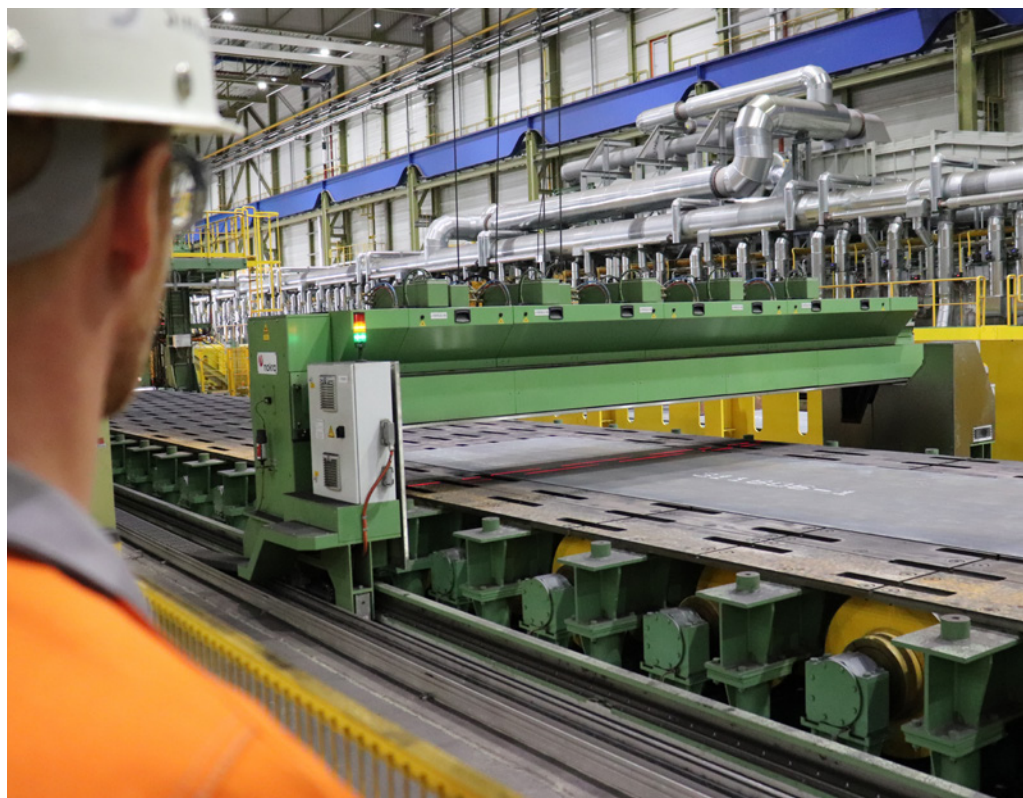
With almost 30 meters in length, the flatness measuring system installed downstream the new RM 5 levelling machine is the largest measuring system ever built by nokra (Picture: Ilseburger Grobblech GmbH)
