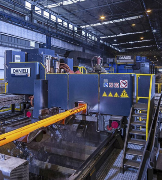
Billet welding machine for endless rolling (Photo: Danieli)
