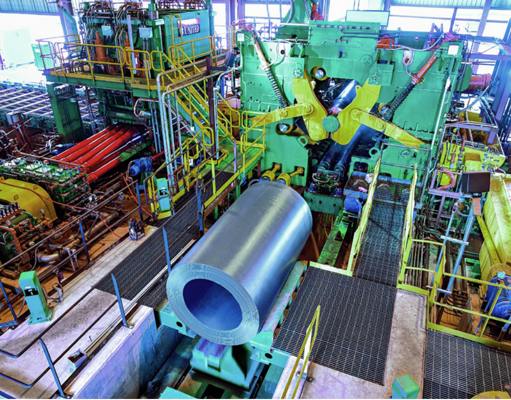
Jumbo coiled plate may way up to 60 short tons (54.4 t) (Picture: Danieli)
