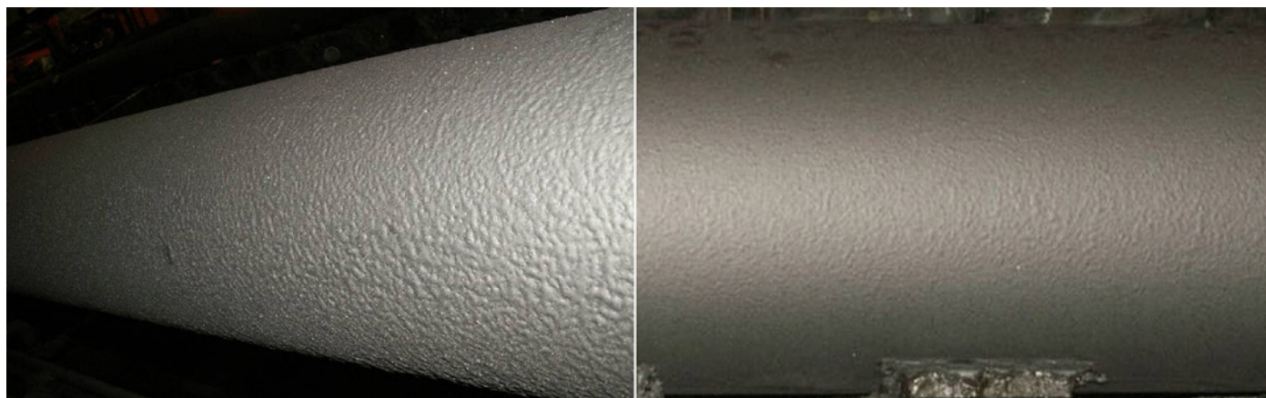
Loose porous standard application (left) compared to a clean tight dry film (right) of ScaleFree coating (Picture: DMK Oy)
