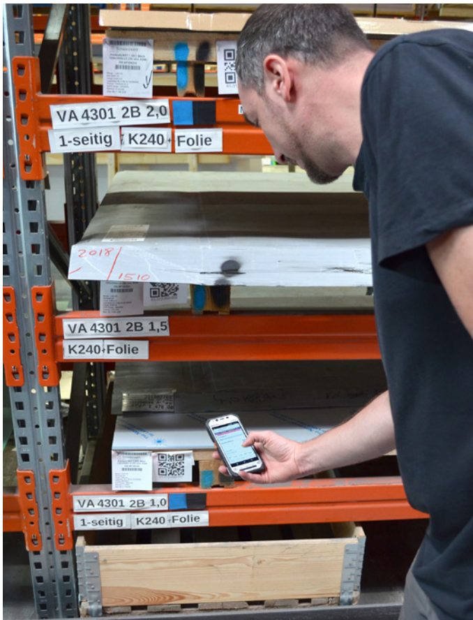
Workers can scan the QR or barcode at the shelves to confirm the removal or trigger a follow-up order (Picture: KASTO)
