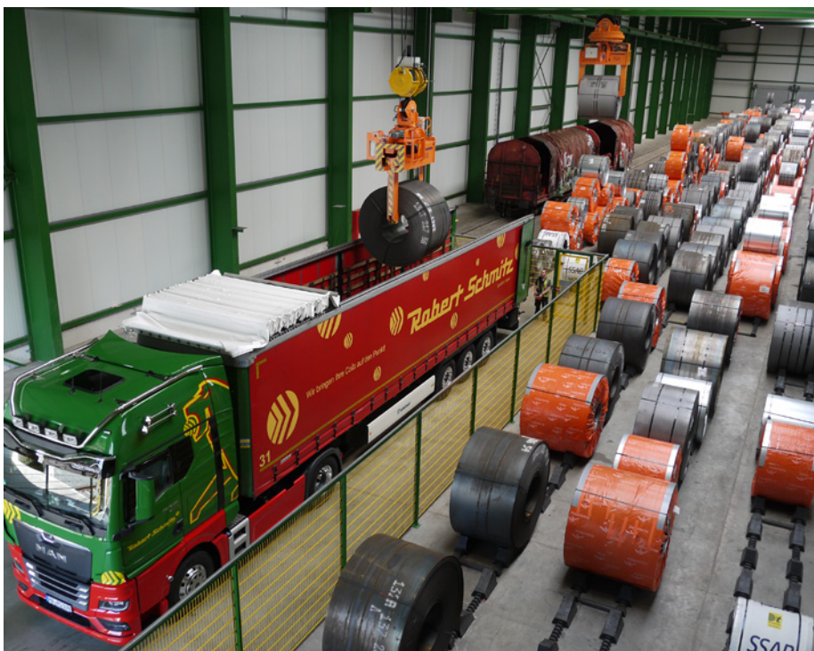
After pre-picking, the coils called up for truck dispatch are stored right by the trucks (Picture: 3tn)
