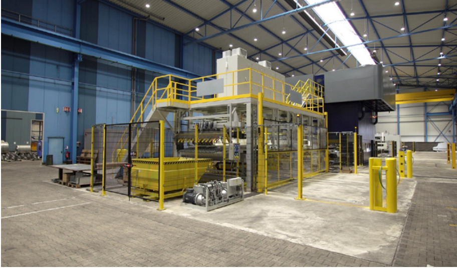
The line's core unit: a high-performance blanking press with capacity of 1,300 t (Picture: Knauf Interfer)
