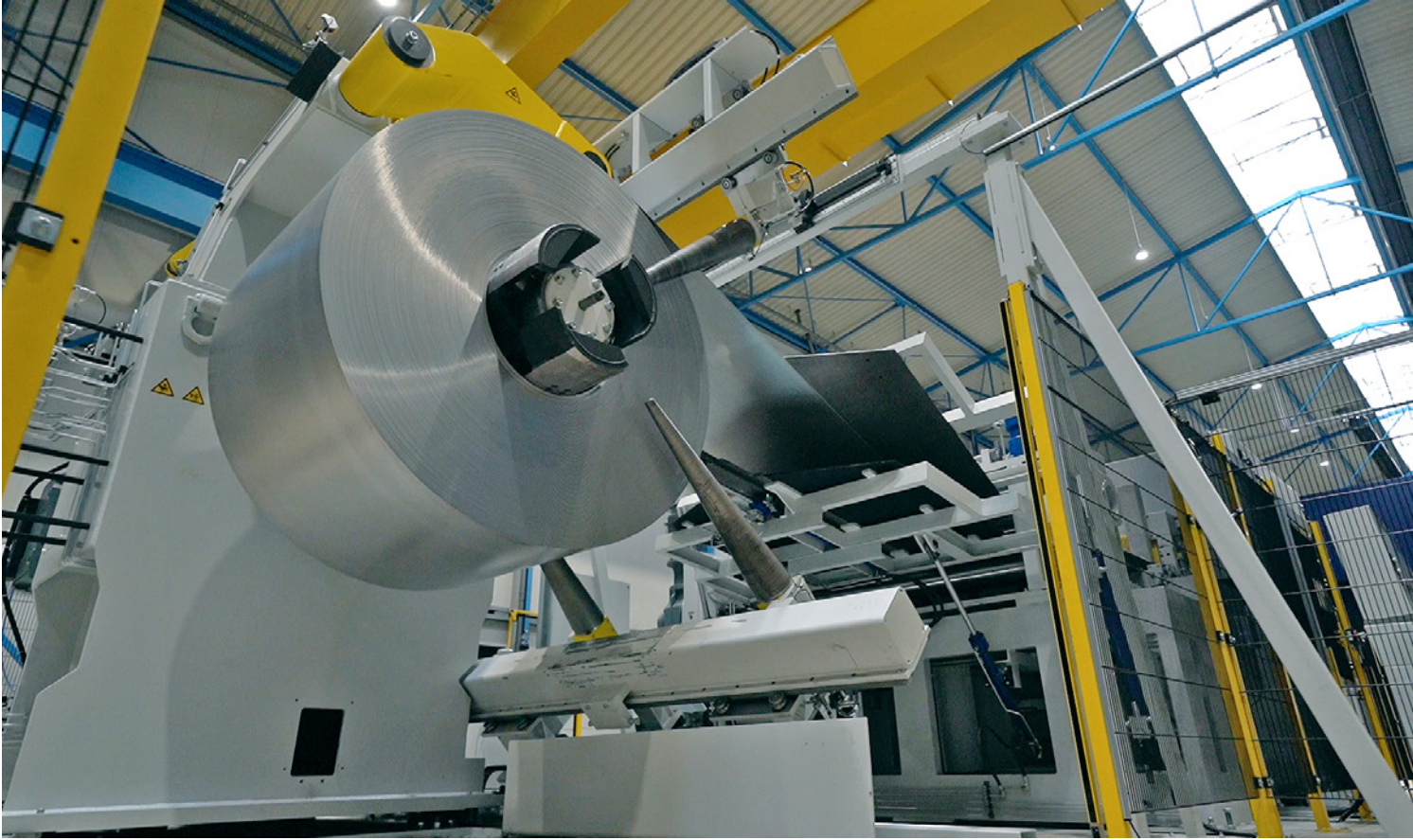
Coils weighing up to 25 t are fed automatically at the entry section of the line (Picture: Knauf Interfer)
