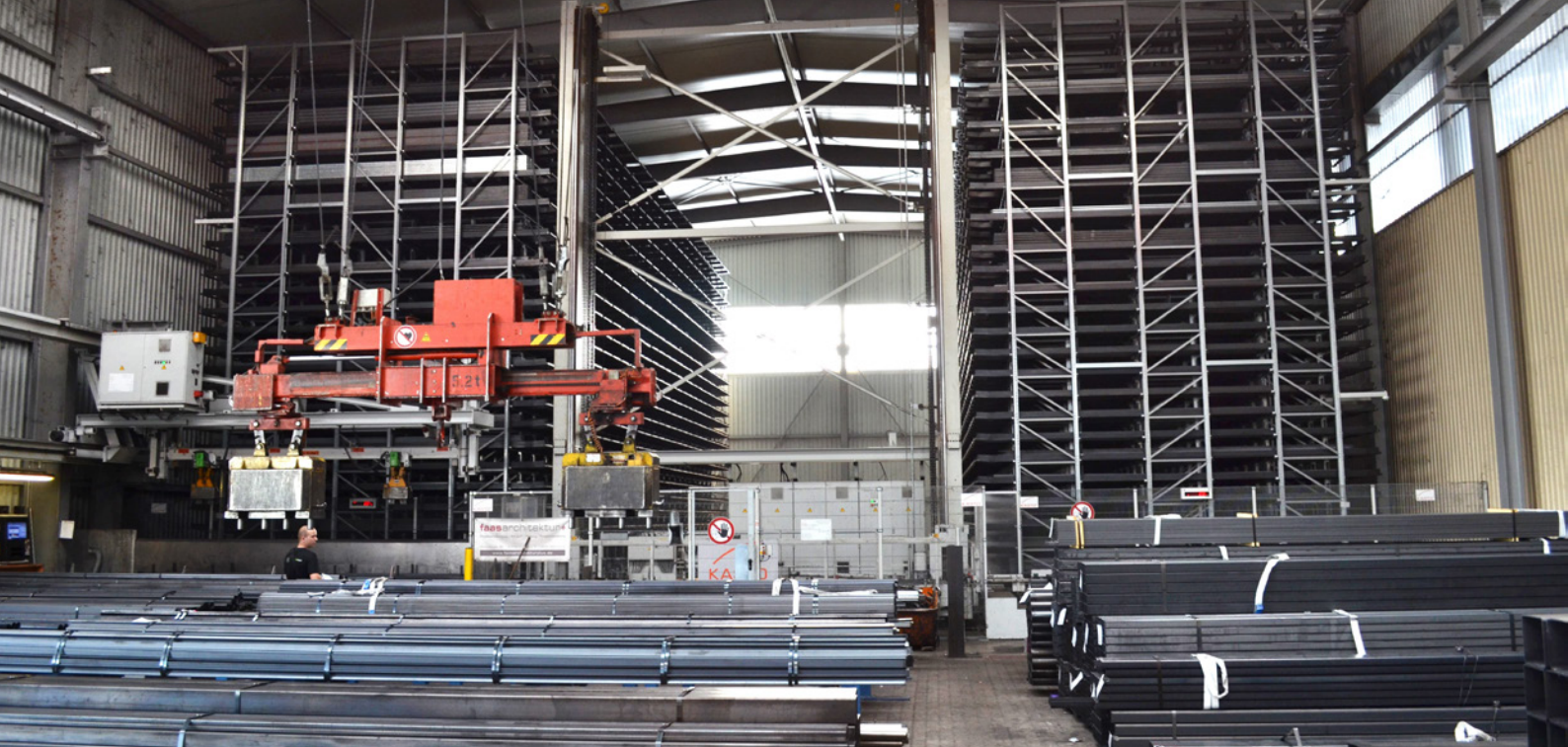
At the company's headquarters, an automated storage system ensures the fast and efficient storage and retrieval of steel products up to six metres long (Picture: KASTO)
