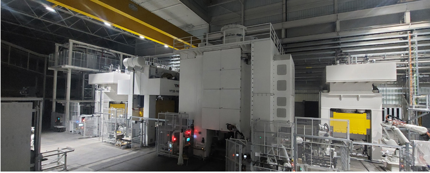
The huge 160 MN forging press (middle) is the centrepiece of the new mechanical forging line (Picture: thyssenkrupp)
