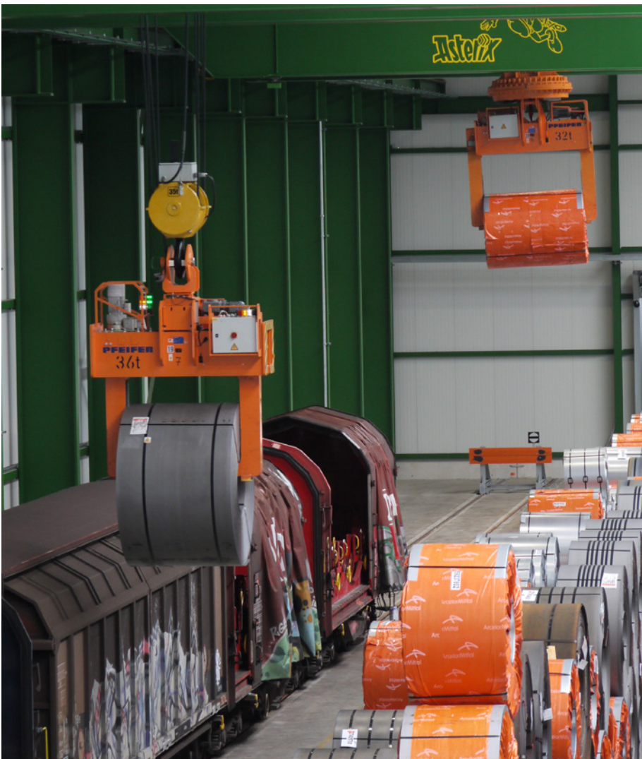
While travelling along the train, Asterix measures the positions, widths and outside diameters of the coils using two 2D laser scanners (Picture: 3tn)
