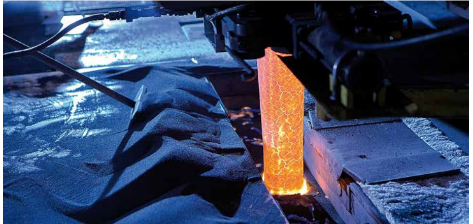
Improved breakout prevention thanks to the new mould control system (Picture: Primetals Technologies)
