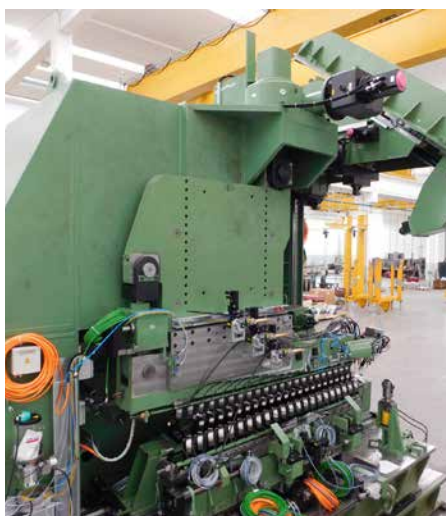
The pipe forming station is the centre-piece of the spiral pipe plant (Picture: SMS group)
