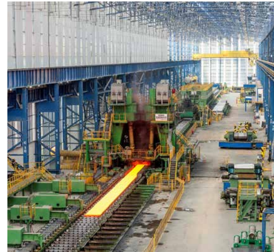
The hot strip mill of Habaş is being expanded to include a further roughing stand (Picture: SMS group)
