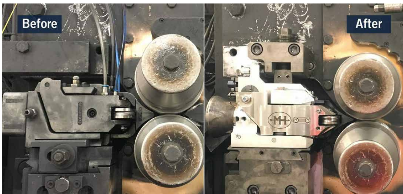
The old and new roller guides installed in the wire rod mill of Gerdau Ouro Branco (Picture: Danieli)
