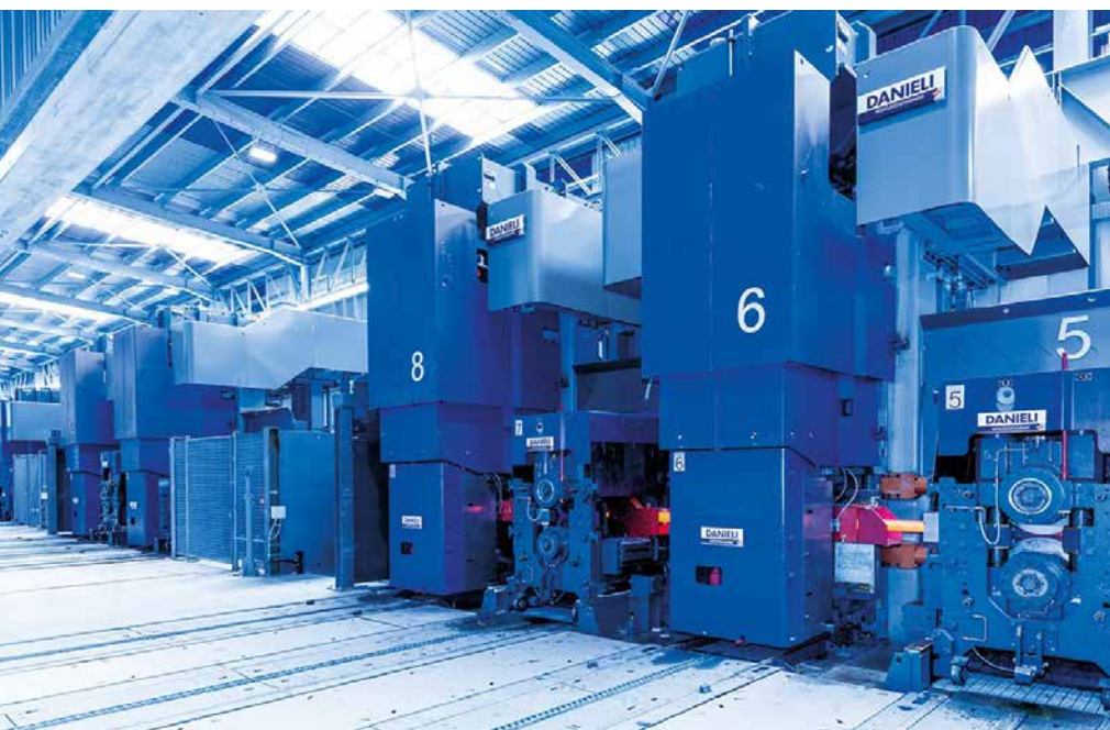
The SHS 4.0 housingless stands are fully electrified to comply with the “Green Mill” concept (Picture: Danieli)
