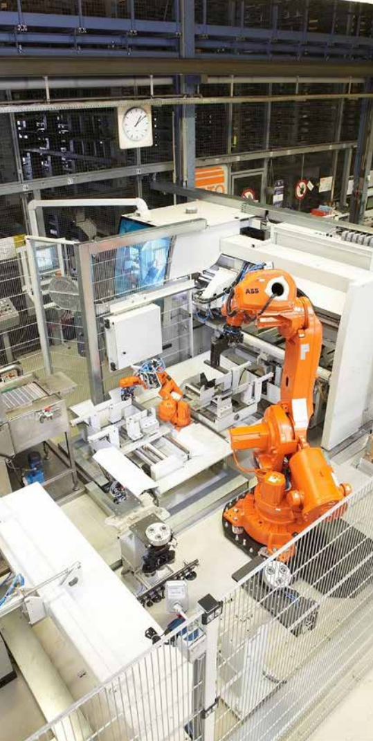
With the robotic handling system KASTOsort, KASTO provides a solution that enables the automation of upstream and downstream manufacturing processes (Picture: KASTO Maschinenbau GmbH & Co. KG)
