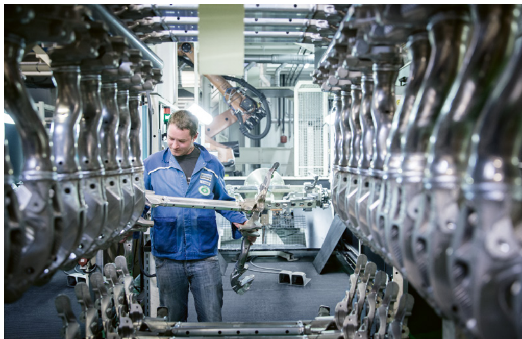
Figure 1. High-strength steels can save weight of chassis components like rear axles (Picture: BENTELER)
