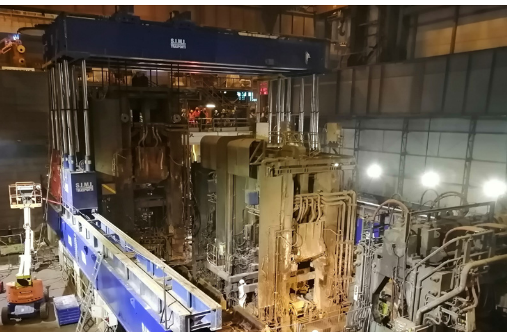
A special crane moves the rolling stand R1 to its new position as R3 in the Arvedi ESP Line (Picture: Primetals Technologies)
