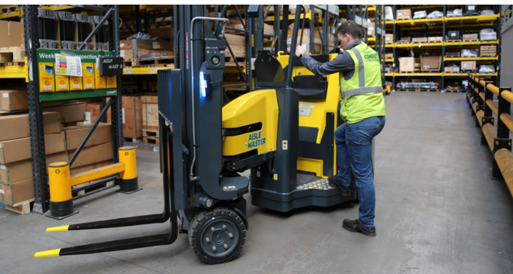
The low floor height of just 280mm enables convenient, single step access from both sides of the truck (Picture: Combilift)
