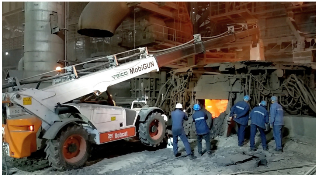
Gunning robot type MobiGUN when gunning an EAF (Picture: VELCO)
