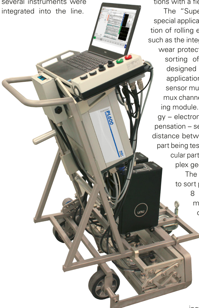
Test trolley ELOTEST HST 3, with 64 sensors for the detection of partial hard spots on heavy plates (Picture: Rohmann)
