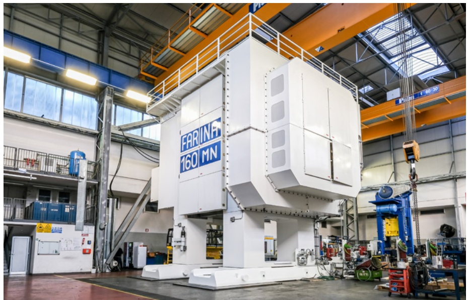
The Farina press lines of the GLF series feature a novel direct drive concept without connecting rods (Picture: Schuler)
