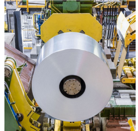
Production of galvanized steel strip in the "heat-to-coat" process (Picture: SMS group)
