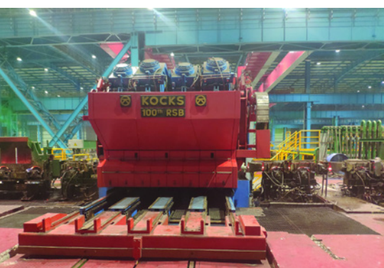
The 100th RSB® reducing & sizing block supplied is in operation at Jiangsu Yonggang (Picture: Kocks)
