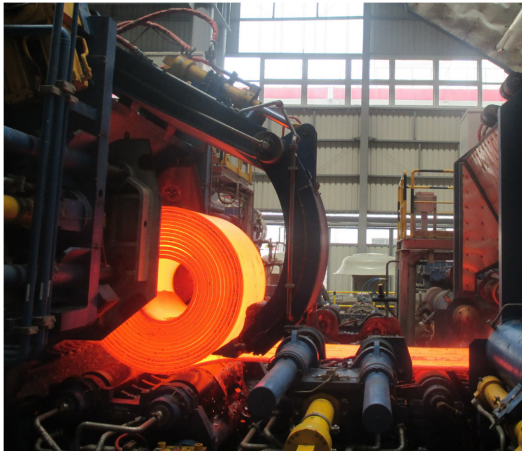
The transfer bar is coiled in the mandrel-less coilbox, where the temperature losses of the inner windings are extremely low (Picture: SMS group)
