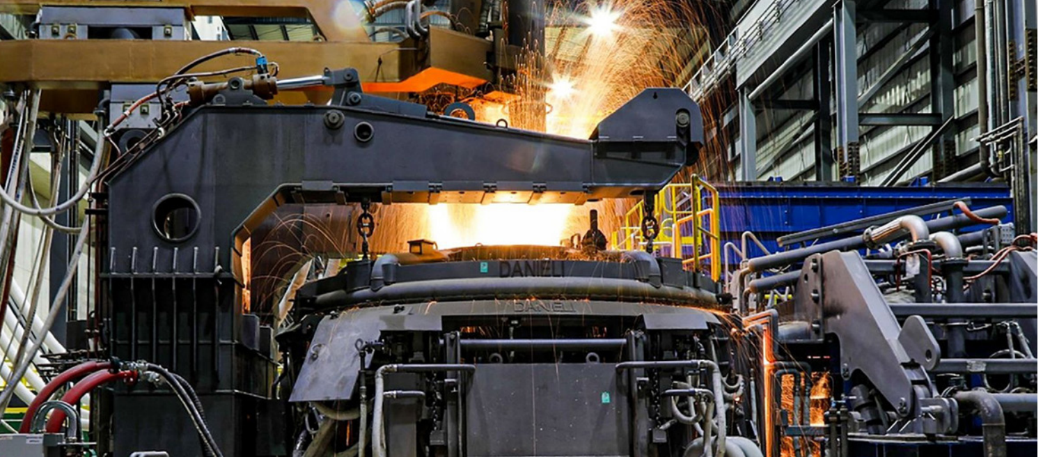
Preheated scrap is charged continuously into the 40-t Fastarc EAF (Picture: Danieli)
