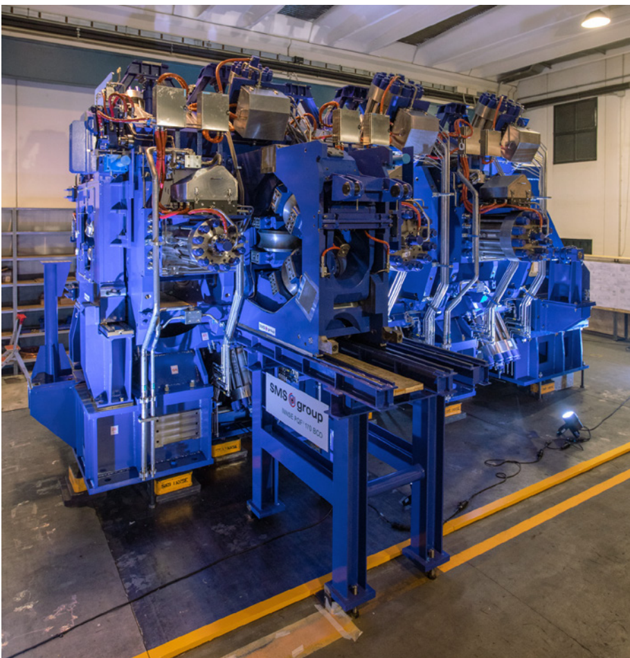
The 4th generation 7-inch PQF® is able to roll 200 tubes per hour (Picture: SMS group)
