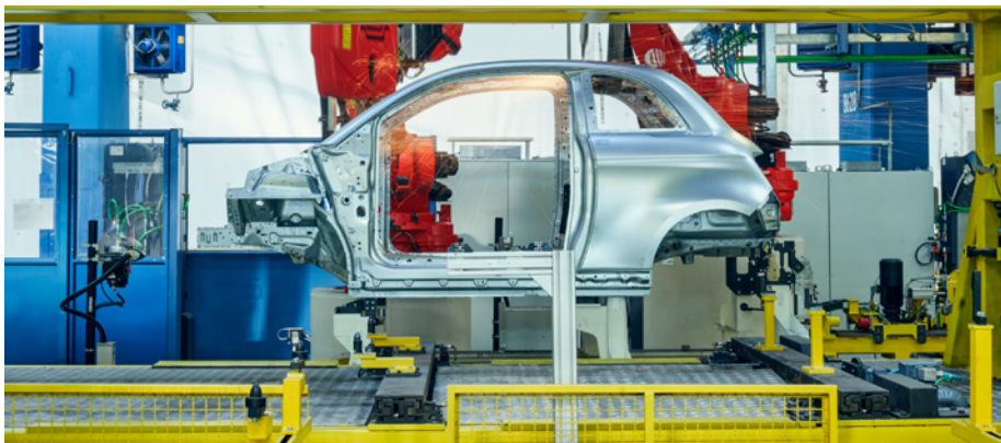
The car body was reengineered to house the battery and transmission of the iconic vehicle (Picture: Comau)
