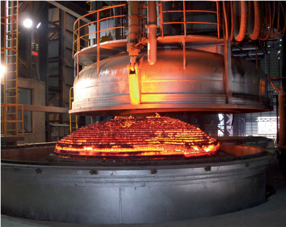
Vacuum treatment in a VOD plant for the refinement of steel for advanced requirements (Picture: Tenova)
