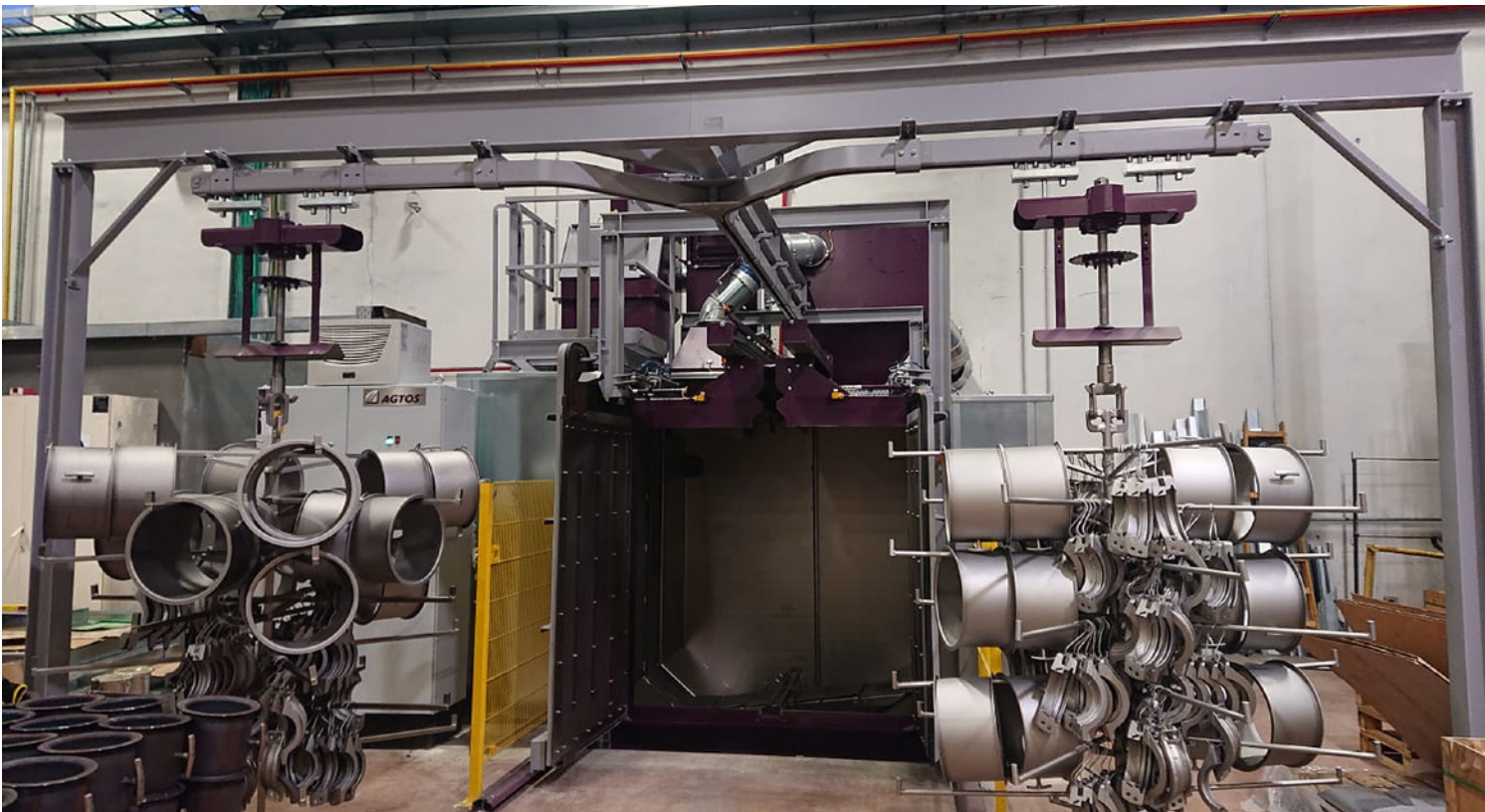
The AGTOS hanger-type blast machine from type HT 17-17 (Picture: AGTOS)
