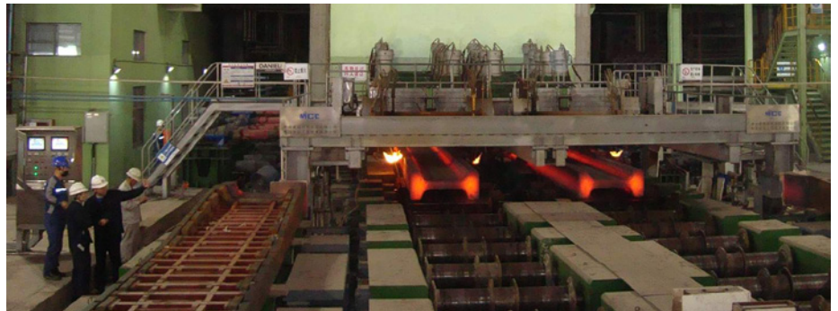
Beam-blank production on the combi-caster at MaSteel (Picture: Danieli)
