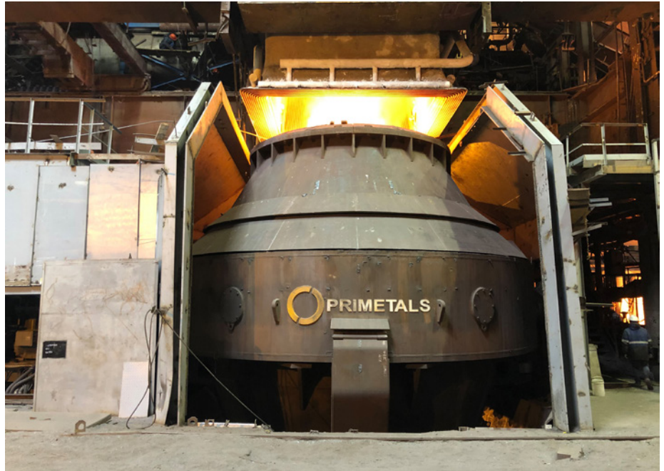
The modernized LD (BOF) converter at the Chelyabinsk Metallurgical Plant (Picture: Primetals Technologies)
