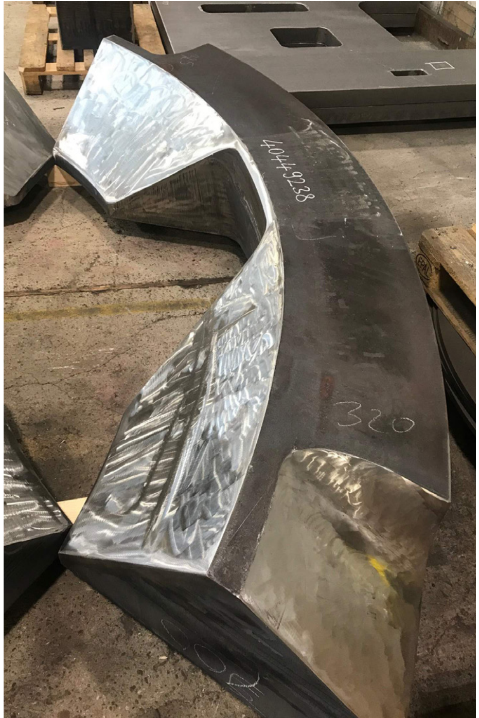
High flame cutting expertise from Jebens in 400-millimetre thickness (Picture: Jebens GmbH)
