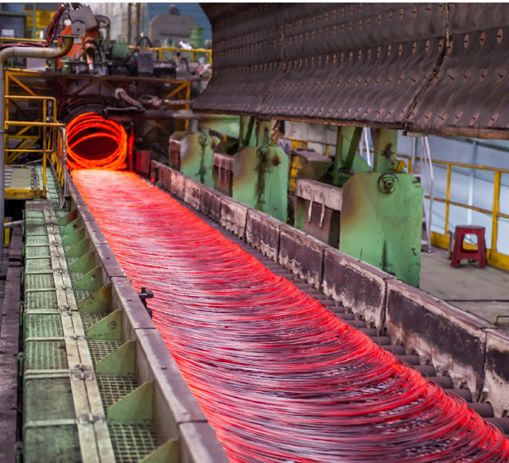
A Morgan Stelmor conveyor in operation during rod production (Picture: Primetals Technologies)
