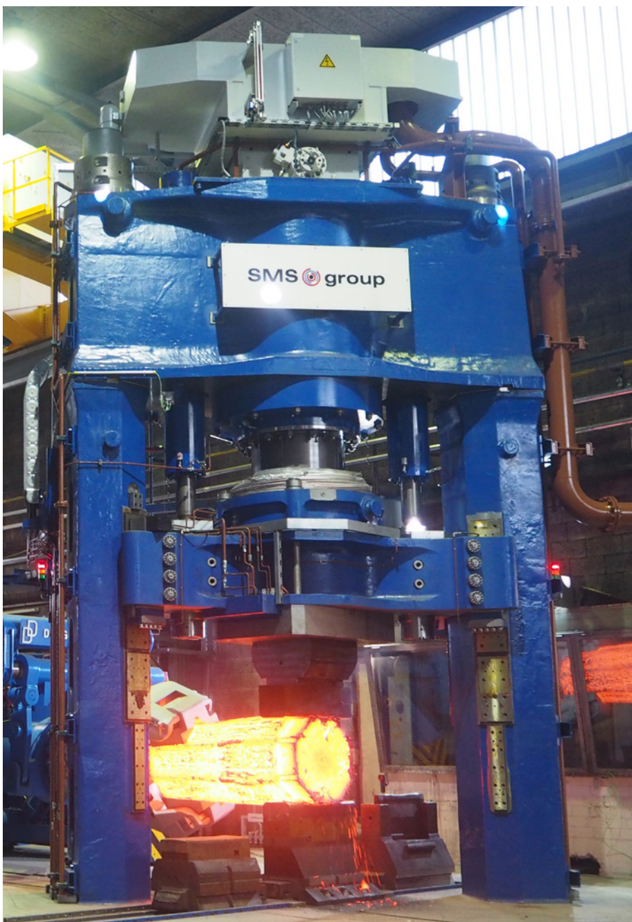
Fig. 1. Forging of the first bloom on the new high-speed press supplied by SMS group to Gustav Grimm in Remscheid, Germany (Picture: SMS group)
