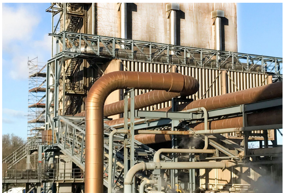
Paul Wurth's cold water granulation system with dynamic INBA® dewatering technique is an officially recognised Best Available Technology (BAT) in the steelmaking industry (Picture: Paul Wurth)
