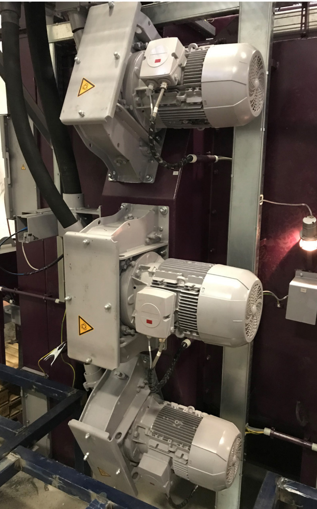
AGTOS turbines with wear parts made of highly wear-resistant hard metal (Picture: AGTOS)
