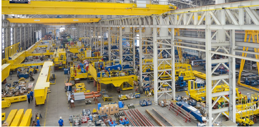
Electric overhead traveling cranes of the type to be installed in the new plate mill of Nucor Brandenburg (Picture: Danieli)
