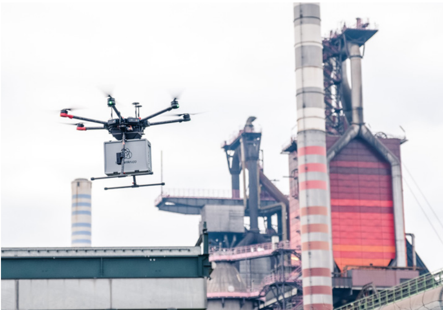
Saves time and protects the environment: Once the transport box is attached to the drone with a patented gripping mechanism, it can be sent to its destination with the push of a button (Picture: thyssenkrupp Steel Europe)
