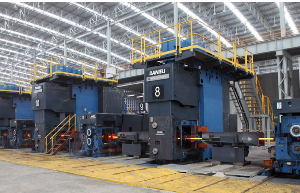
Rolling stands of a bar and light-section mill (Picture: Danieli)
