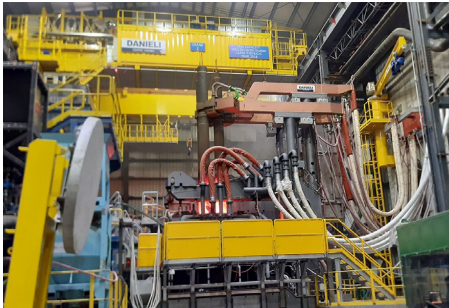
Electric arc furnace of the new MiDa endless casting-rolling minimill at Nucor Steel Sedalia (Picture: Danieli)
