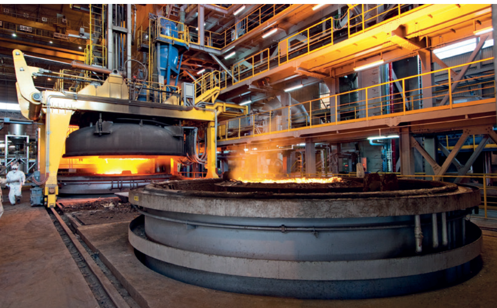
Figure 1. Twin-tank VD station (Picture: Danieli)
