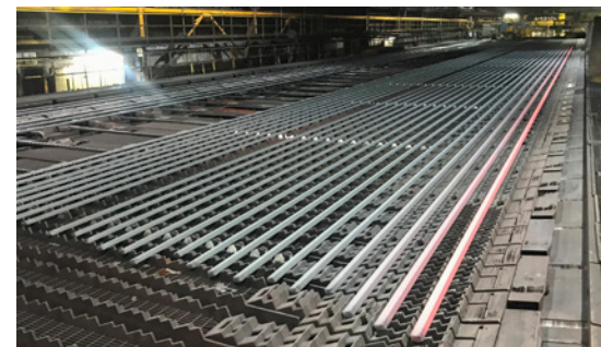
The automation upgrade covered the production chain down to the cooling bed (Picture: AIC Automazioni Industriali Capitanio)
