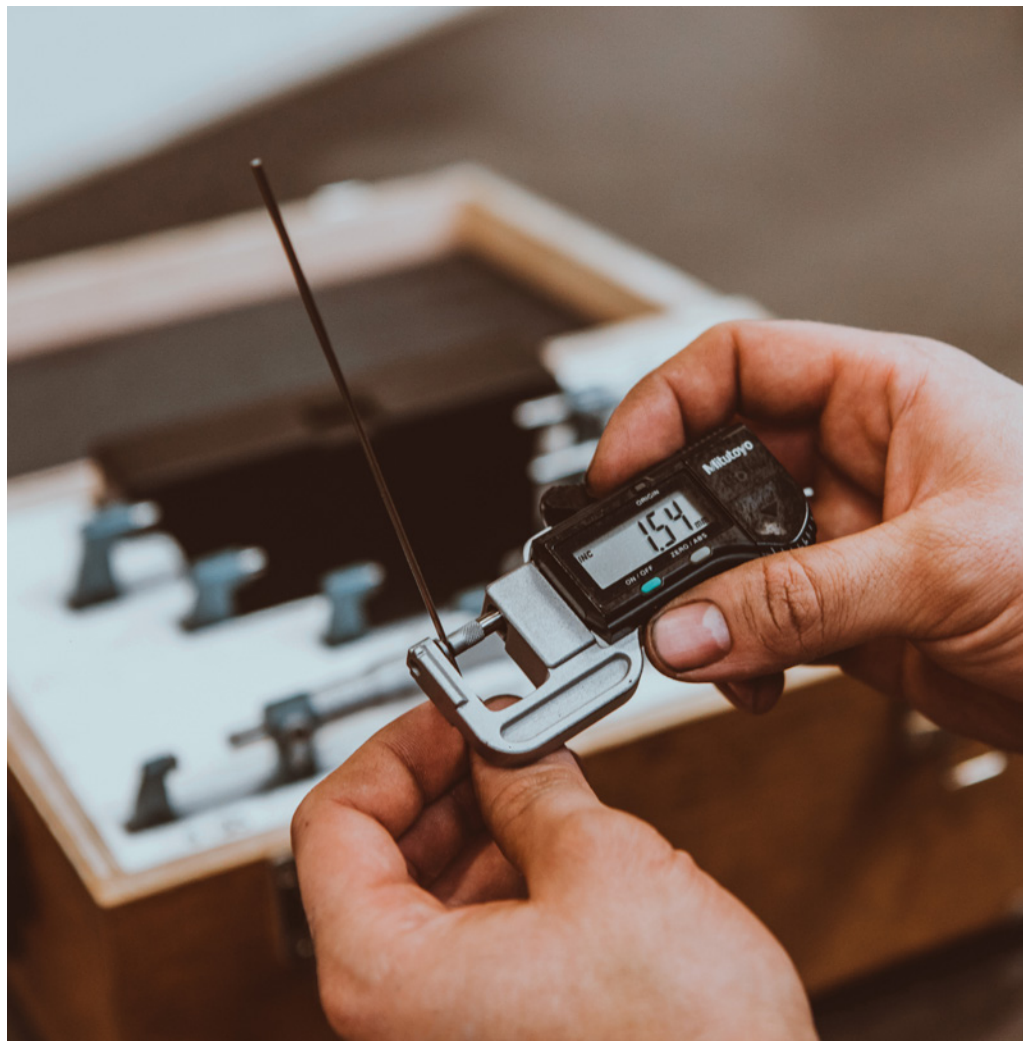
The new machine produces double thick end spokes with a diameter of only about 1.5 mm in the middle (Picture: AMBA)
