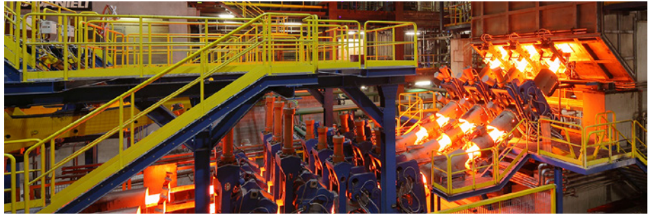
A casting machine for blooms will be installed at Chengde Jianlong (Picture: Danieli)
