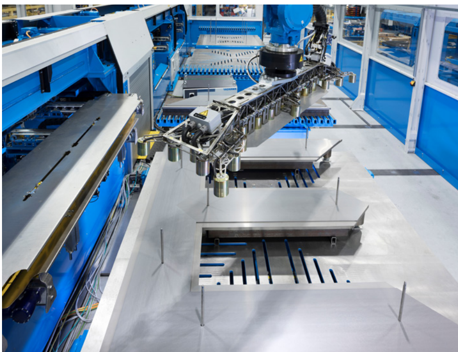
The robot removes the cut laminations from the punching and cutting unit, transports them to the stacking area and stacks the lamination cores fully automatically and with highest accuracy of repetition (Picture: GEORG)
