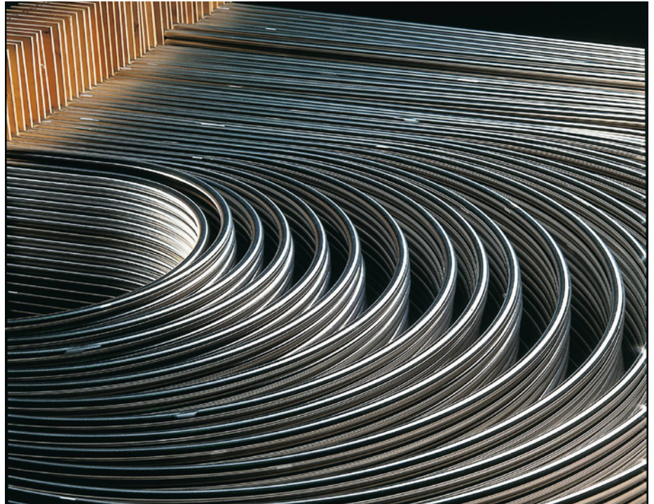
U-bent tubes for heat exchangers (Picture: Sandvik)
