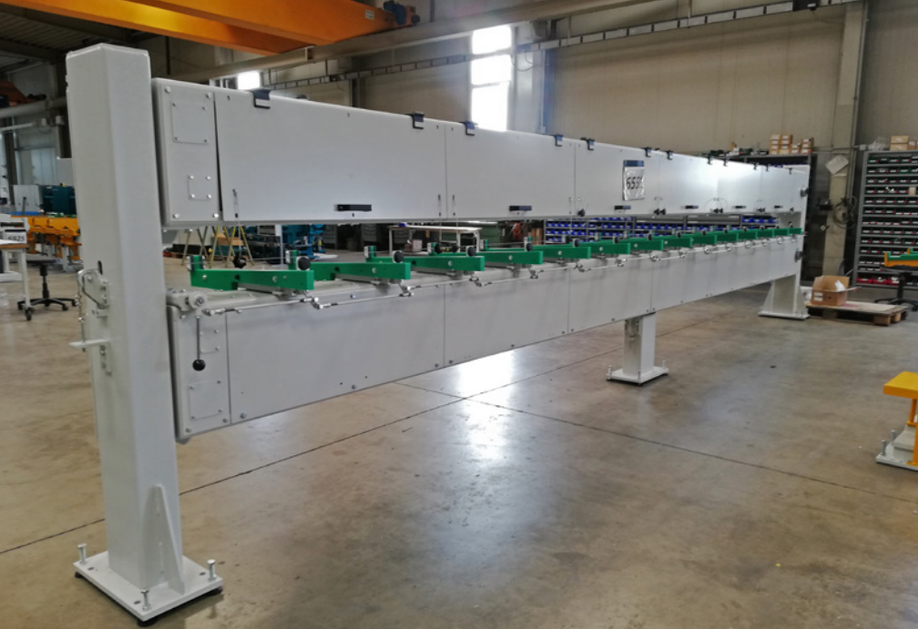
A gauging system ready for shipment to the customer; the measuring frame is only 30 cm wide (Picture: sema Systemtechnik)
