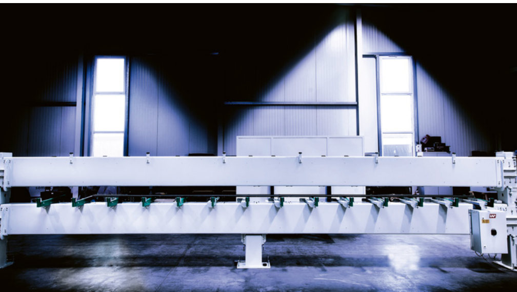
The gauge can be equipped with up to 16 sensors, as requested by the customer (Picture: LAP)
