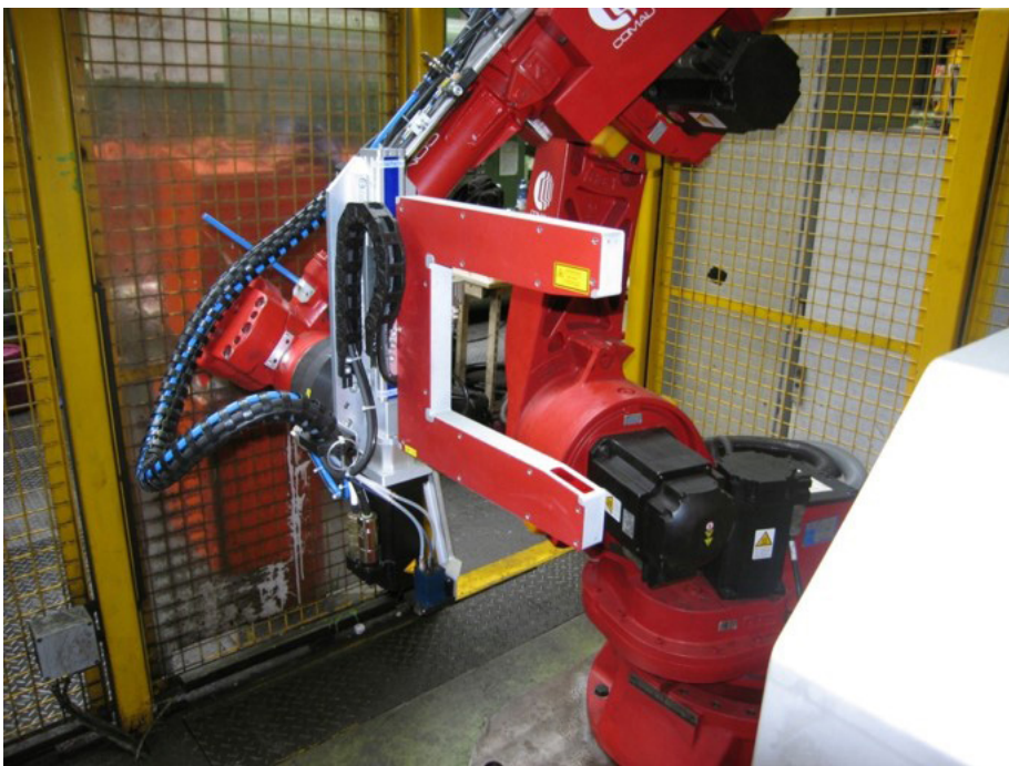
The robot to the side of the roller conveyor extends its arm with sensors from the protected parking position into the tube end, and scans the entire tube circumference through 360° (Picture: LAP)
