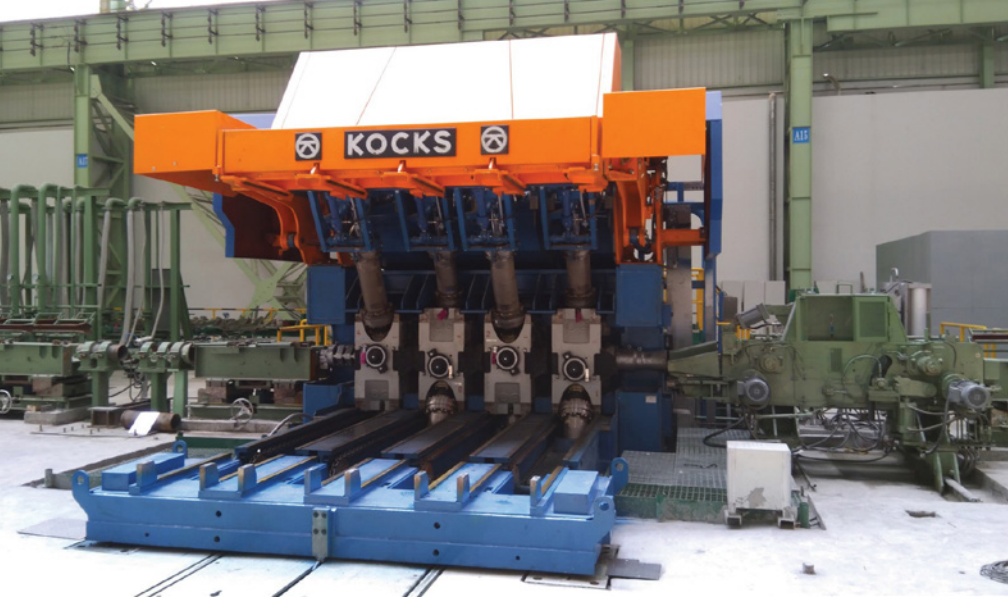
With the new reducing-sizing block, Shaoguan intends to increase SBQ production (Picture: Friedrich Kocks)
