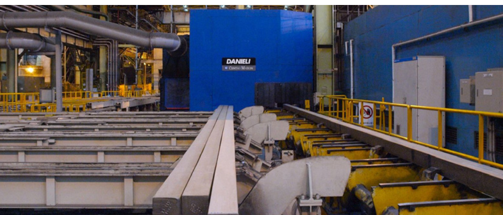
The new grinders will be designed for 150 mm square billets (Picture: Danieli)
