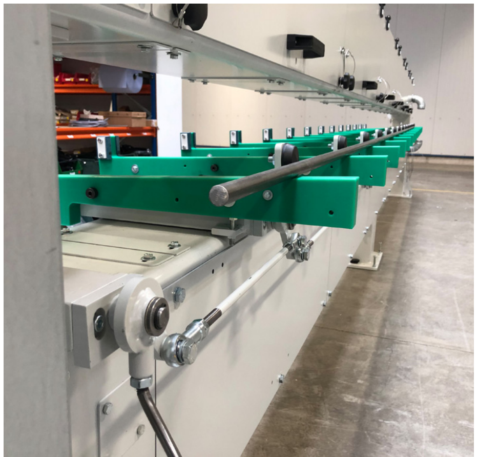
Rounds roll through the measuring frame over a slide; the lasers are arranged in the upper part, the receiving optics in the lower part of the measuring frame (Picture: sema Systemtechnik)
