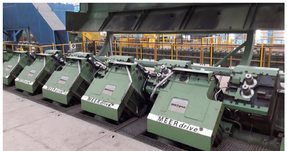
Figure 6. MEERdrive® block (Picture: SMS group)
