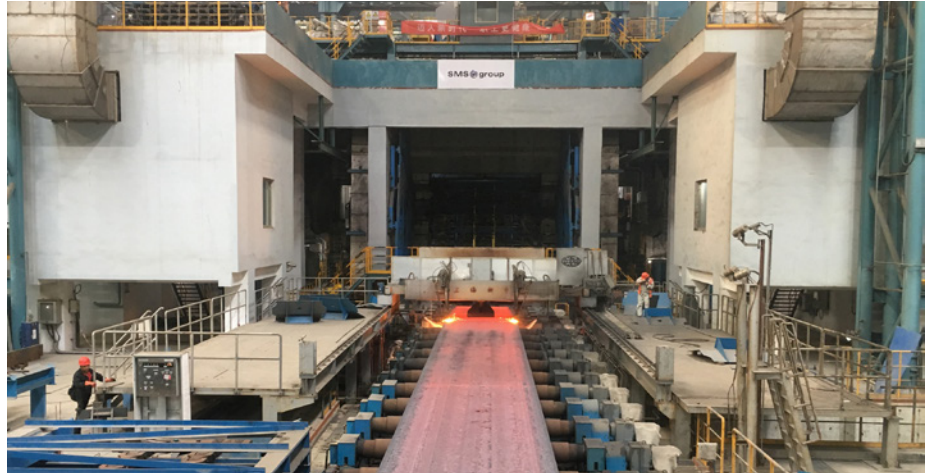
First slab produced on the new casting machine at Shandong Rizhao (Picture: SMS group)
