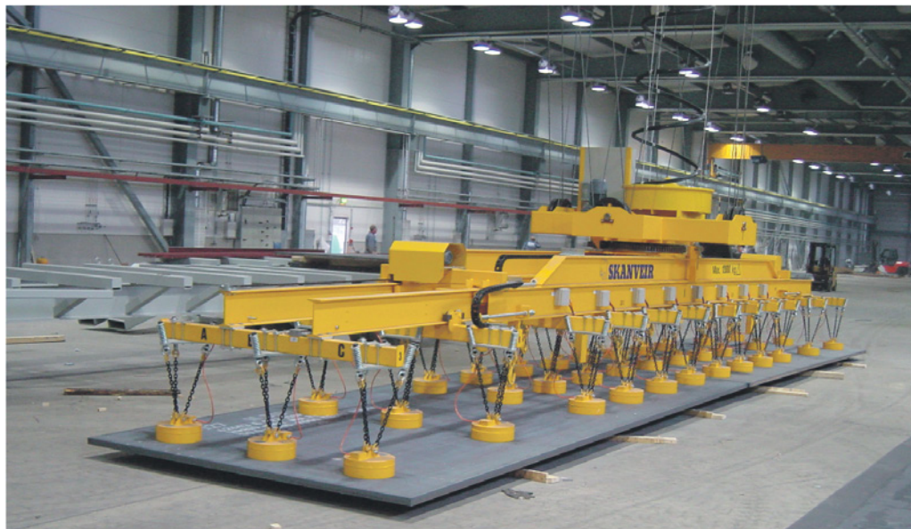
Skanveir magnetic beam with motorised telescopes allows quick and safe handling of different plate sizes (Picture: Skanveir)
