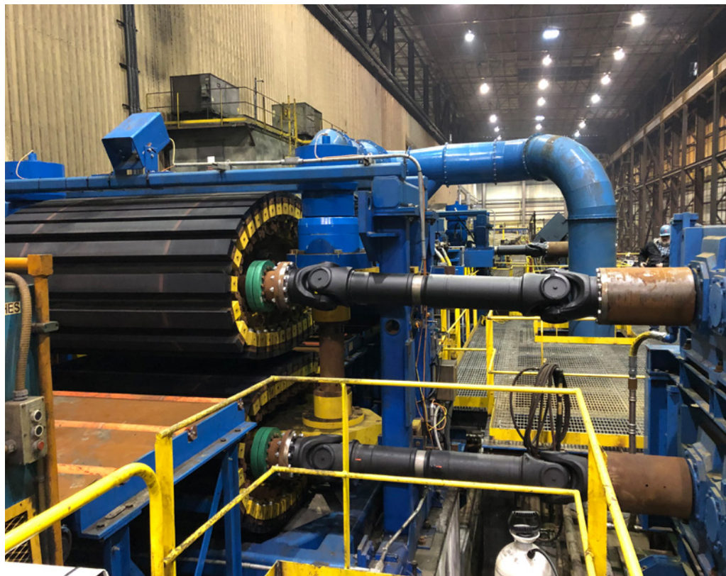
Entry section of the BTU Umlauf Bridle (Picture: SES Engineering)
