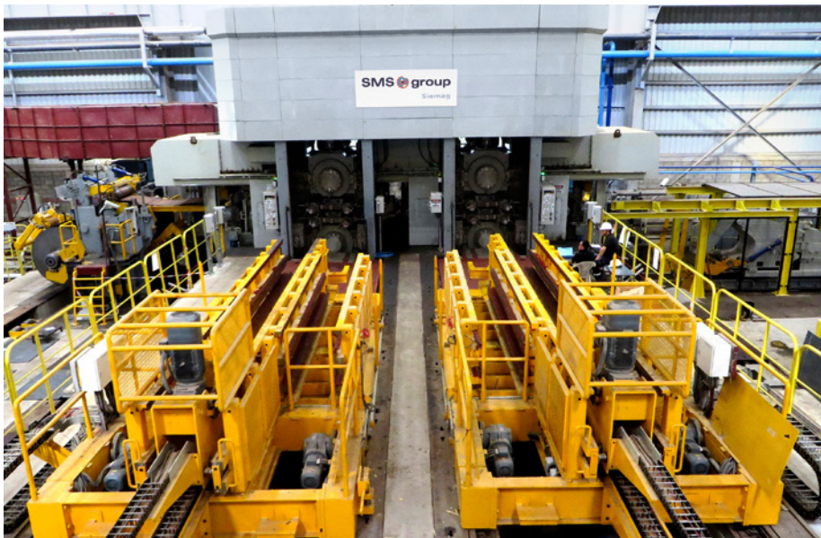
Overview of the CCM® provided with two four-high mill stands, entry- and exit-side as well as roll change equipment (Picture: SMS group)
