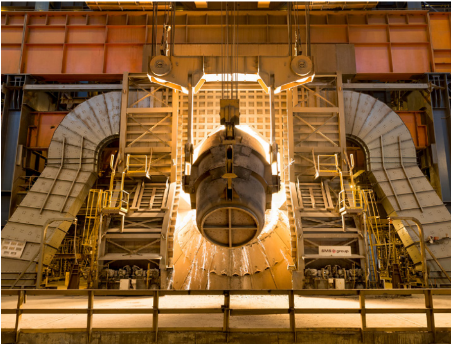
BOF converter equipped with maintenance-free lamella suspension system of the type supplied to SAIL (Picture: SMS group)
