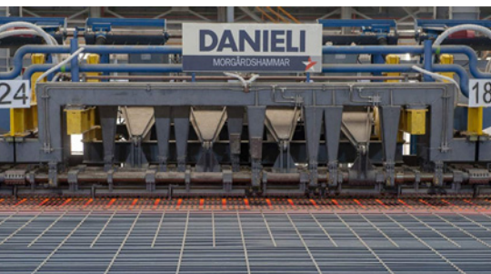
High-speed rebar rolling mill (Picture: Danieli)
