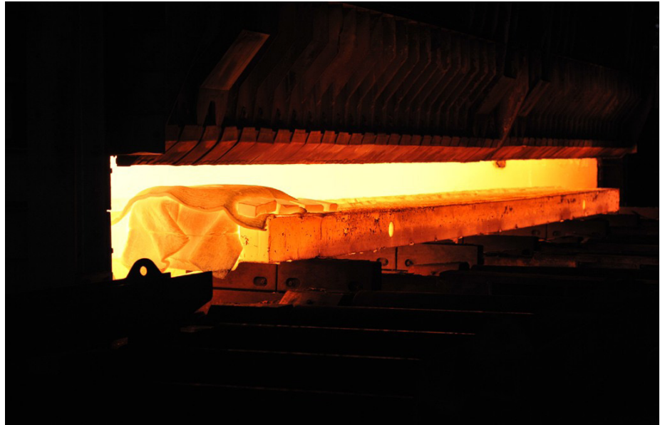
Figure 2. Monitoring a steel slab being reheated prior to hot rolling (Figure: PhoenixTM)
