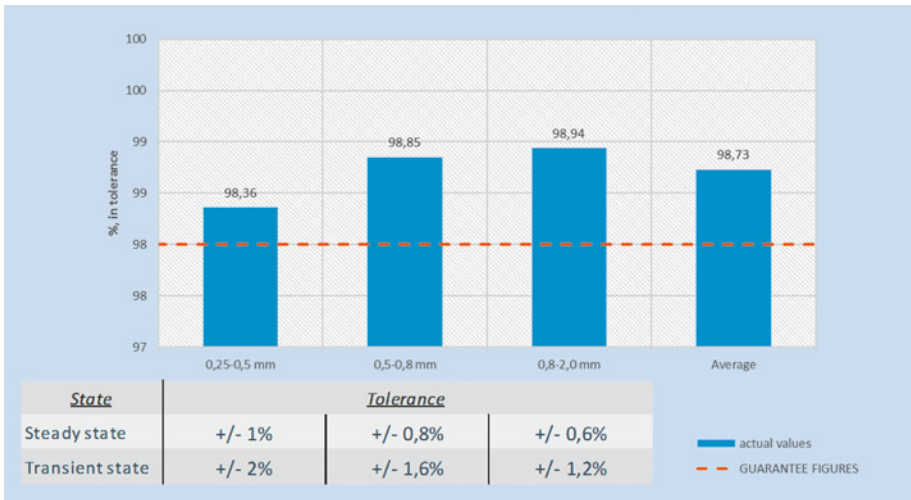
Achieved thickness performance (Picture: Danieli)
