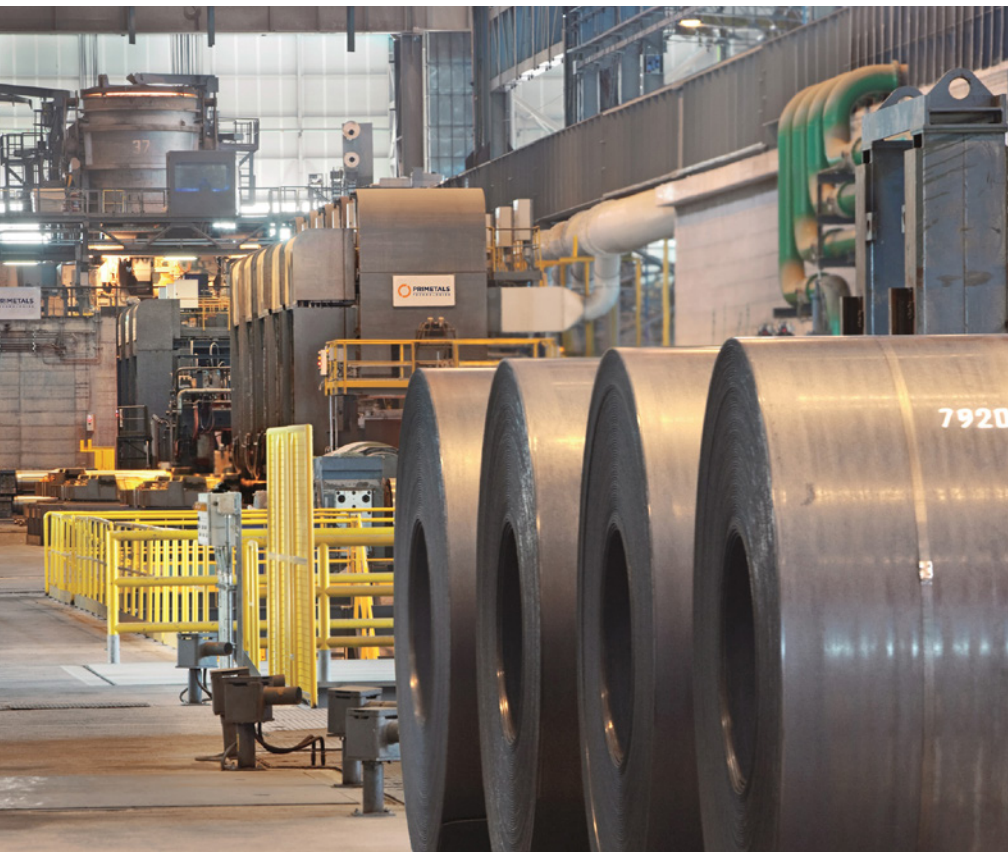
Arvedi Endless Strip production lines directly link casting and rolling (Picture: Primetals Technologies)
