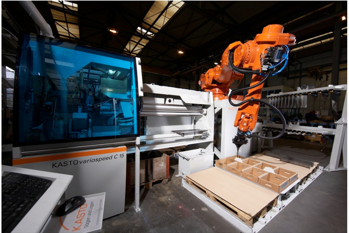
With the Kastosort robot link, the removal of the saw cuts can be automated, together with a wide range of other tasks like deburring, chamfering, centring, threading, marking, printing, sorting, stacking and picking (Picture: Kasto Maschinenbau GmbH & Co. KG)
