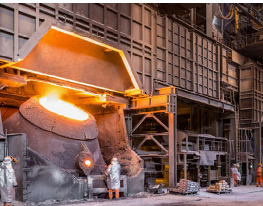
BOF converter meltshop of HBIS Serbia where Primetals Technologies will replace converter No. 2 (Picture: HBIS)
