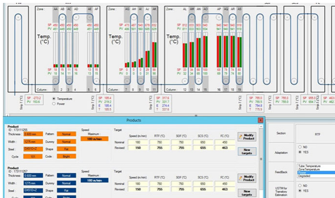
HMI of the thermal optimization system for processing lines
