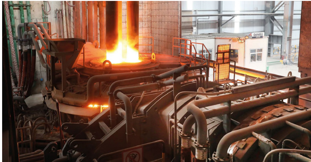
The first Zero-bucket EAF in China is in operation at Guihang Metal products (Picture: Danieli)
