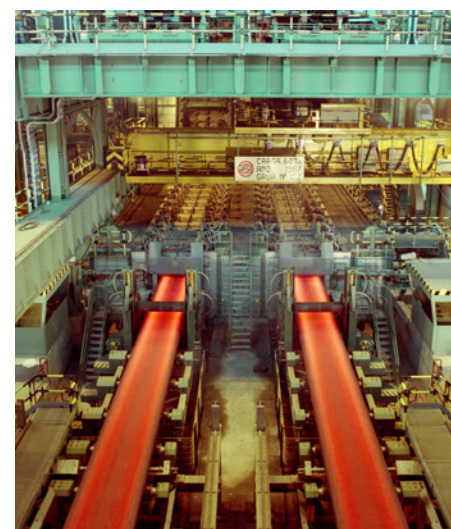
ArcelorMittal Asturias, Spain, Continuous casting line, Avilés steel shop (Picture: C. Gutiérrez ©Copyright: ArcelorMittal)
