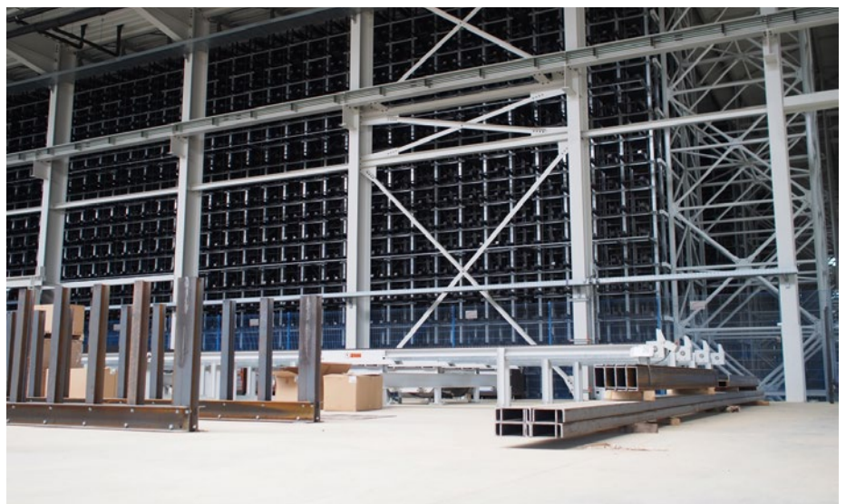
The new „unicompact“ honeycomb warehouse provides more than 10,000 cassettes (Picture: Kasto Maschinenbau GmbH & Co. KG)
