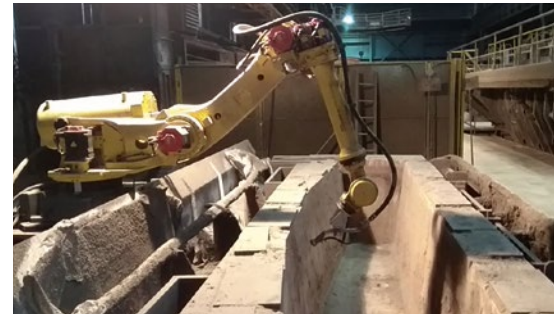
Robotic tundish lining process developed by steel mill team of Trinec Iron and Steel (Picture: Trinec Iron and Steel)
