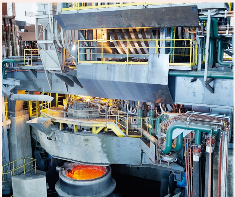
An EAF Quantum electric arc furnace in operation (Picture: Primetals Technologies)
