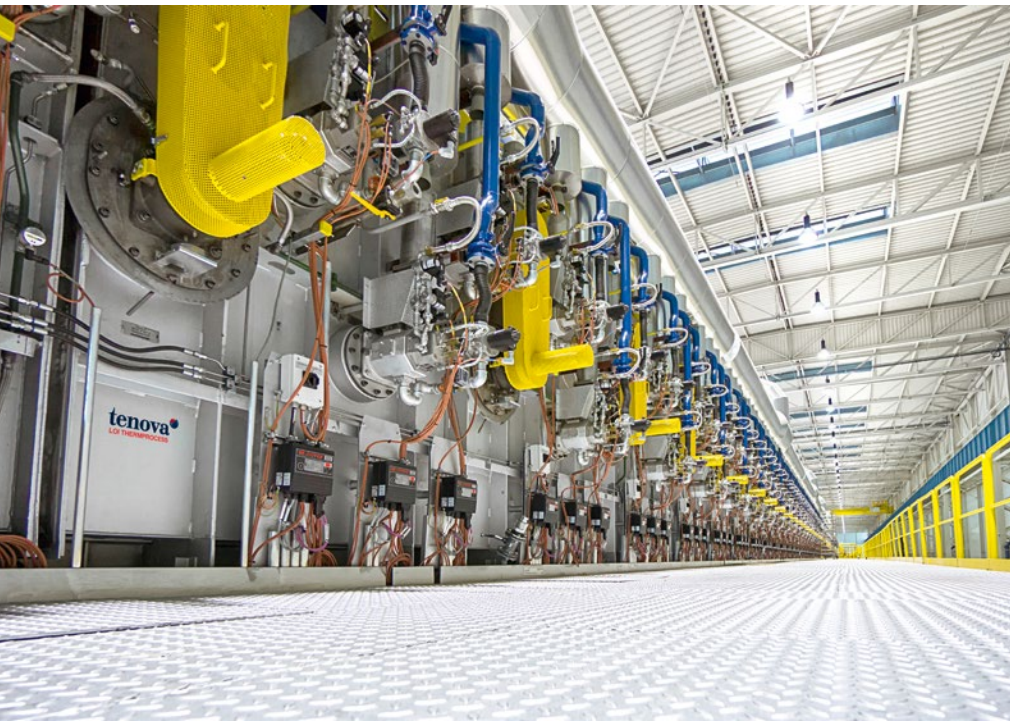
Modern ACL-Line for heat treatment of non-grain-oriented electrical steel (Picture: Tenova LOI Thermprocess)
