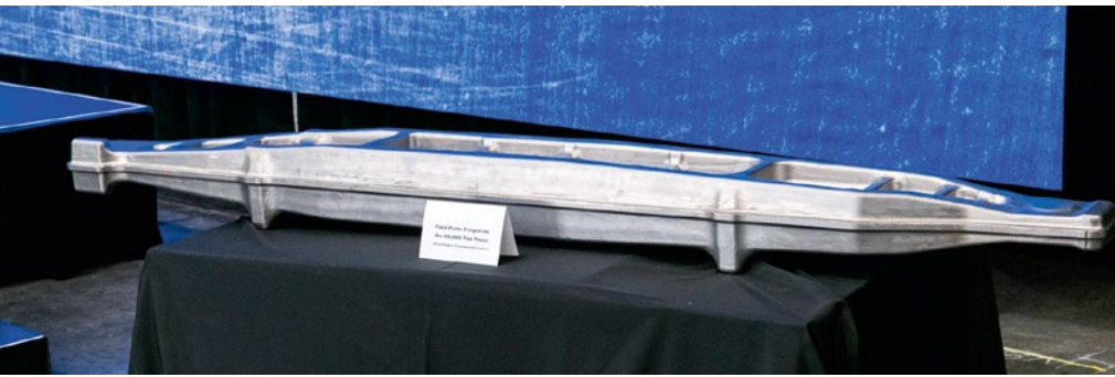
One of the first parts forged on the new die forging press (Picture: SMS group)
