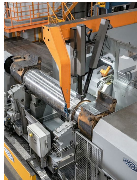
By using CBN abrasive tools, the roll grinding machine reduces grinding times by more than 50 percent (Picture: Heinrich Georg Maschinenfabrik)
