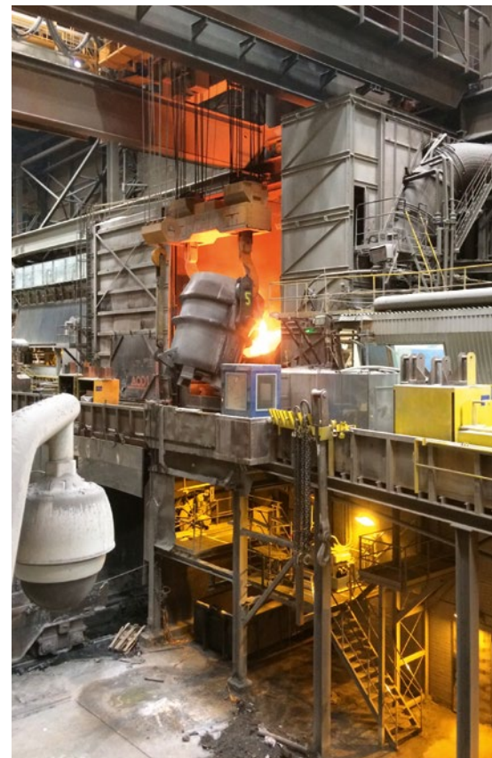
Modernized AOD converter at Outokumpu Stainless Oy in Tornio, Finland (Picture: Primetals Technologies)
