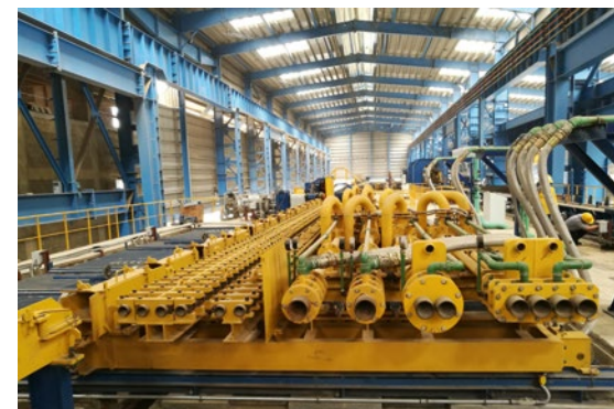
A PQS inline quenching system will be integrated into the new mini-mill for rebar production (Picture: Primetals Technologies)
