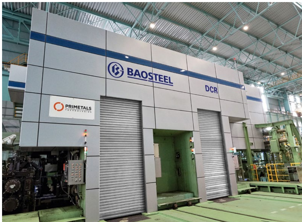
Front view of Baosteel's new double cold reduction mill (Photo: Primetals Technologies)
