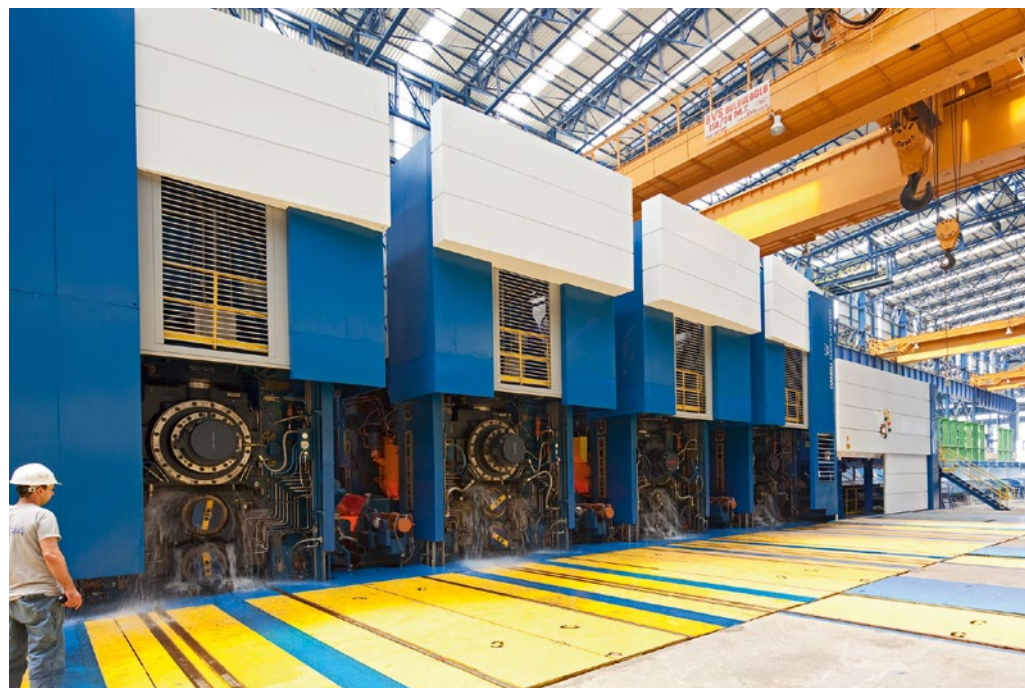
Finishing stands of the QSP hot strip mill under operation at MMK Atakas, Turkey (Picture: Danieli)
