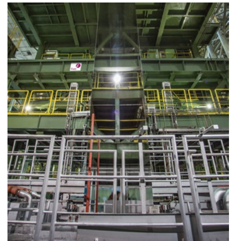
Continuous hot-dip galvanizing line in operation (Picture: Fives)
