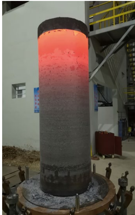
Remelted ingot produced in the ESR furnace (Picture: INTECO)
